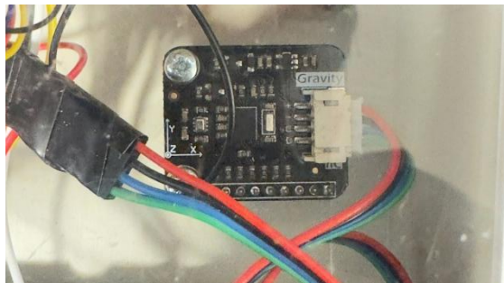
Figure 14: The mounted IMU inside the control box
