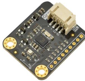
Figure 10: Gravity 10 DOF IMU used for the control box
