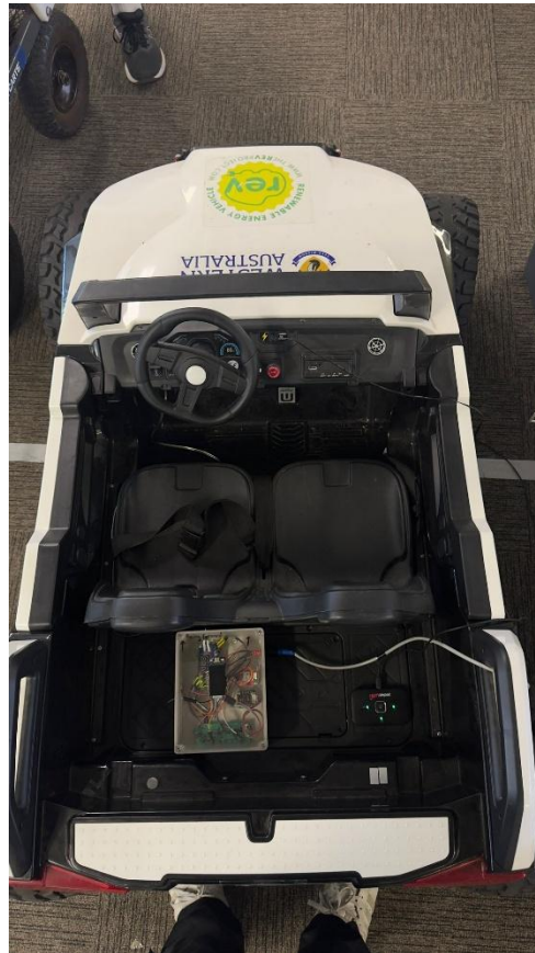
Figure 17: Shows the control box mounted behind the seats of the open top car to provide clear signal for the GPS antenna
