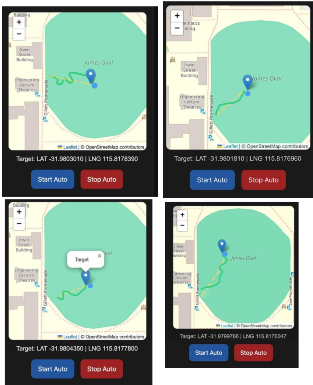
Figure 23: Webservice interface during autonomous waypoint navigation trials at James Oval, showing live GPS position tracking, user-defined target waypoints, and recorded vehicle navigation paths during autonomous operation.
