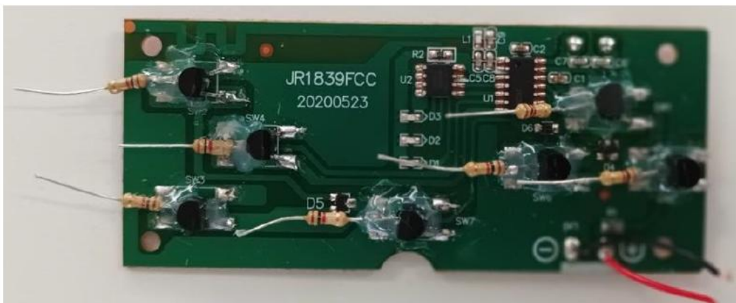
Figure 6 shows the modified remote controller PCB that was used in the project
