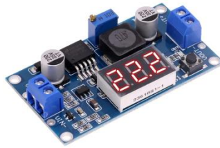
Figure 7 LM2596 DC-DC voltage convertor
