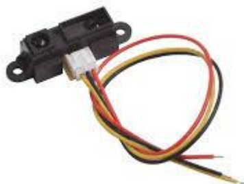
Figure 11: The SHARP PSD sensors used for the project
