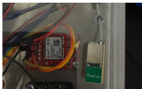
Figure 16: The GPS and then antenna mounted on the control box
