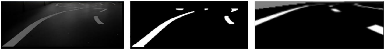
Figure 3.3: The Sim-to-Real visual preprocessing, transforming the raw physical feed (left) into clean track features (middle) that highly resemble the ideal simulation environment (right).
