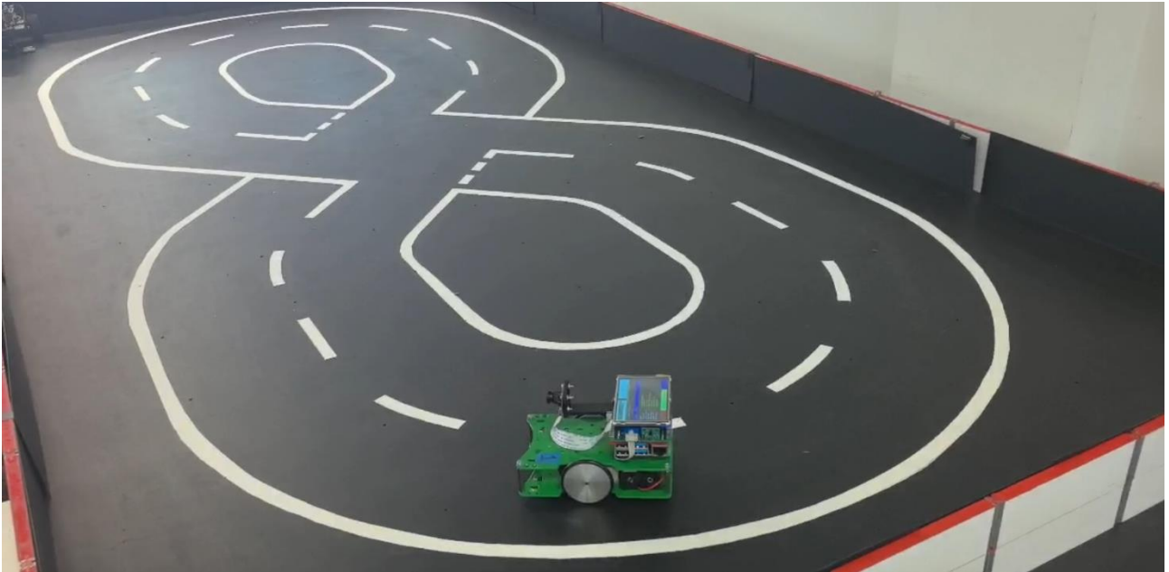
Figure 4.1: The physical laboratory track and the EyeBot robot used for real-world testing, exhibiting visible surface glare and lighting interference.
