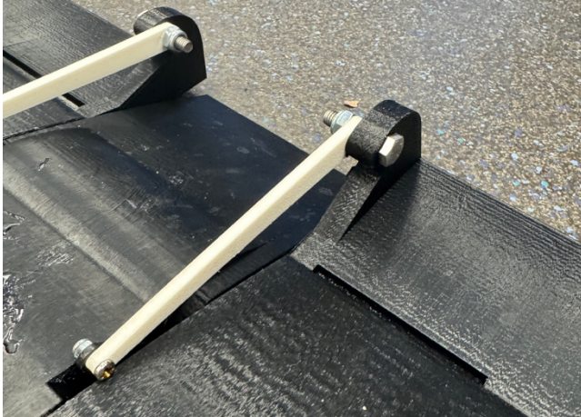
Figure 24 Aileron-Servo Horn Connection Rod
