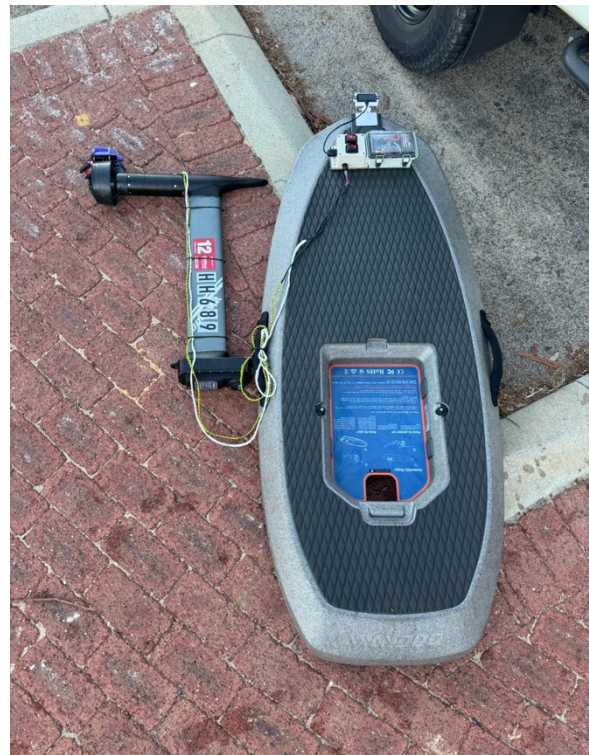
Figure 28 Electrical Assembly Mounted To Board
