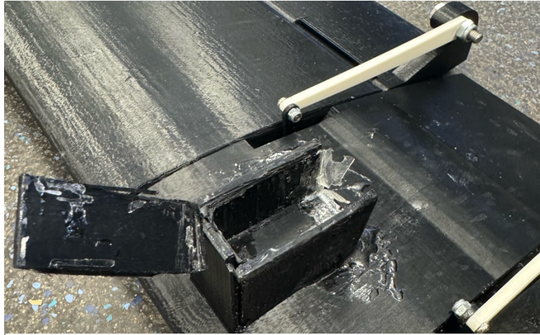
Figure 34 Wing Mount Failure
