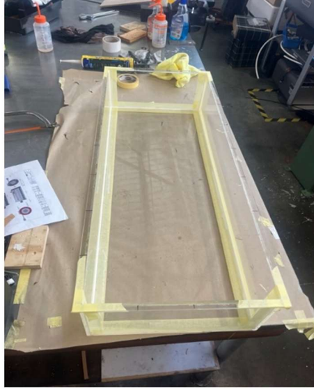
Figure 5.8. UWA engineering workshop applying silicone to internal panel joints
