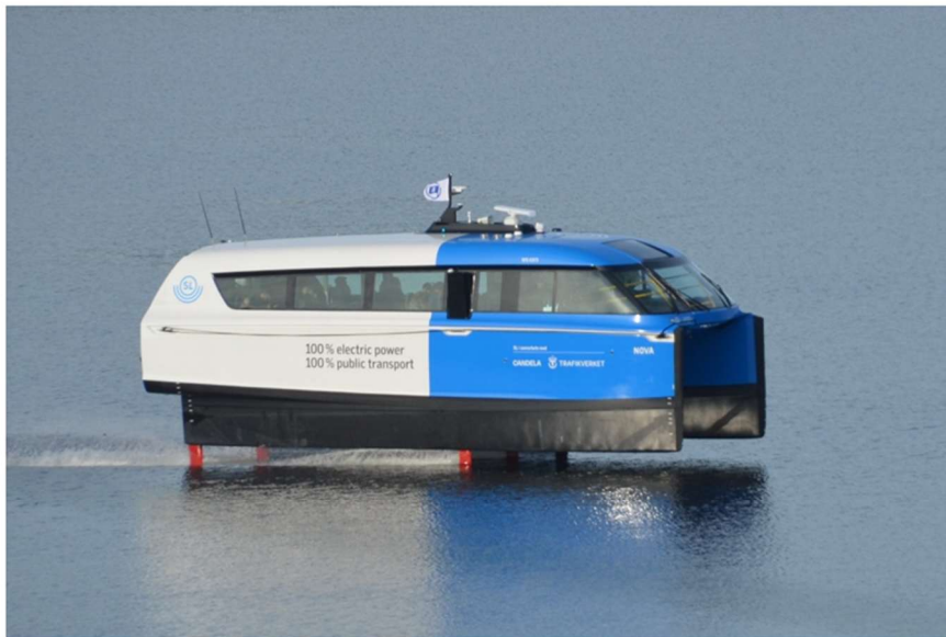
Figure 2.1: Candela P-12 Shuttle operating in foil-borne mode, demonstrating commercial electric hydrofoil passenger transport (Candela, 2024).
