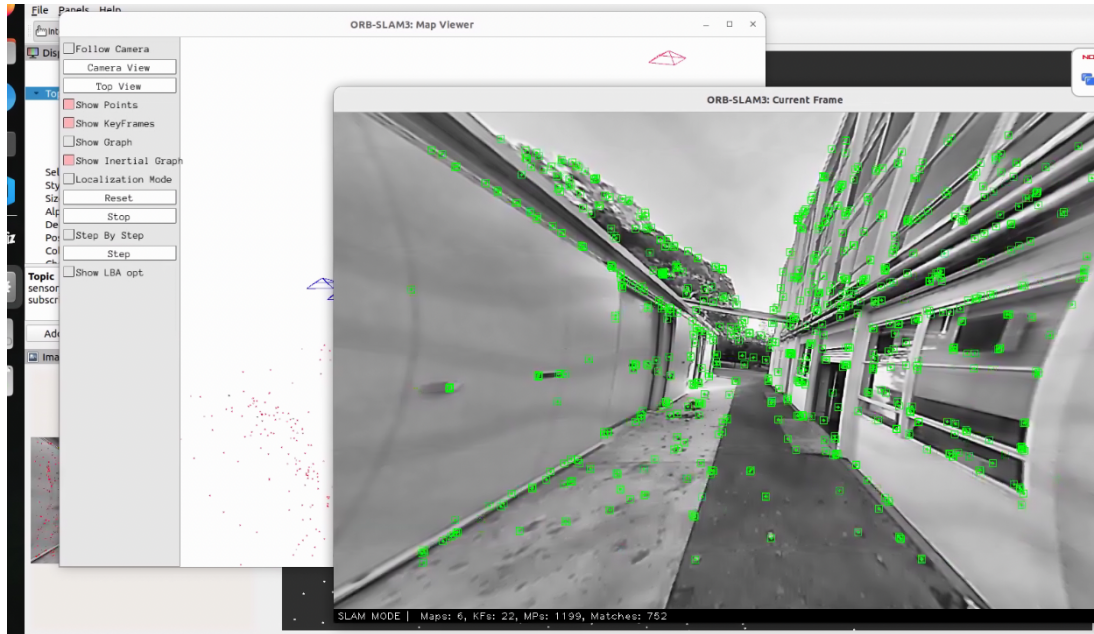
Figure 1.3: ORB keypoints (green squares) detected on a rectified nUWay4 fisheye frame.
