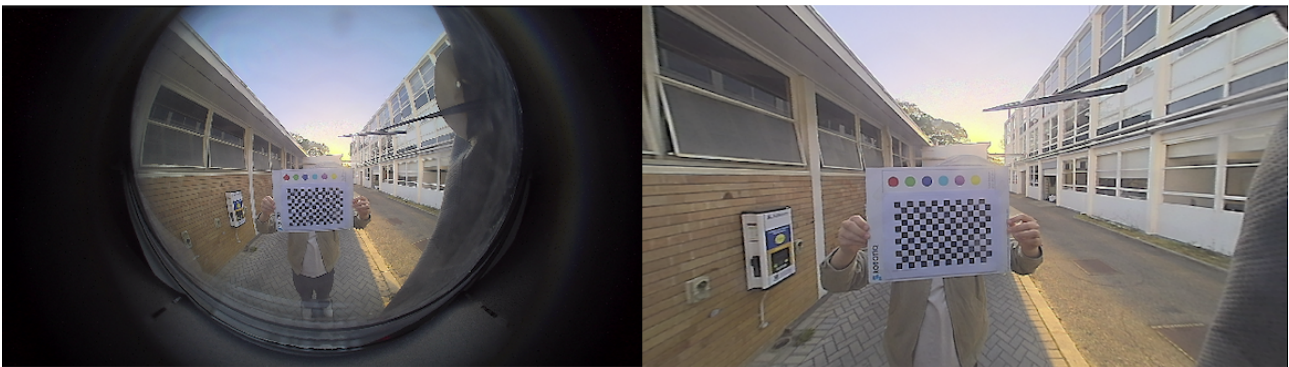
Figure 2.6: GMSL2 fisheye frame before (left) and after (right) calibration and rectification to a pinhole model.
