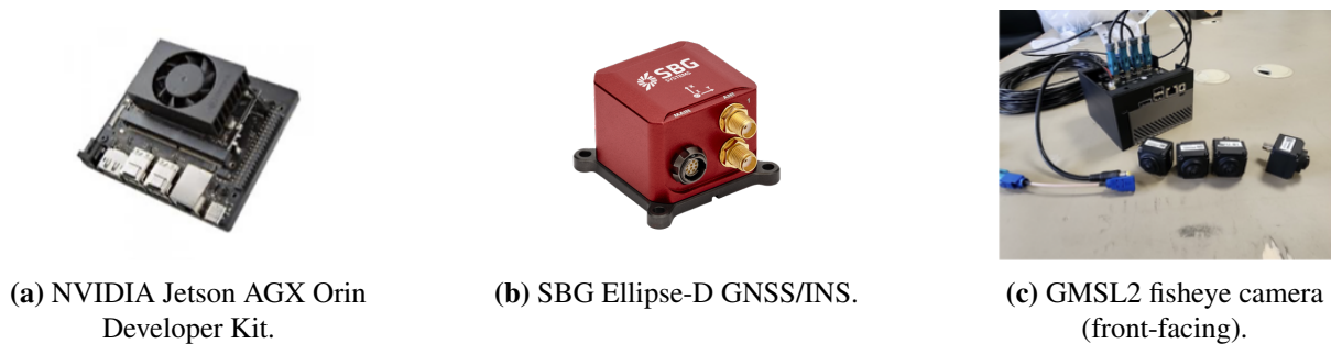
Figure 2.2: Hardware components of the deployed pipeline: Jetson AGX Orin (left), SBG Ellipse-D (centre), GMSL2 fisheye camera (right).
