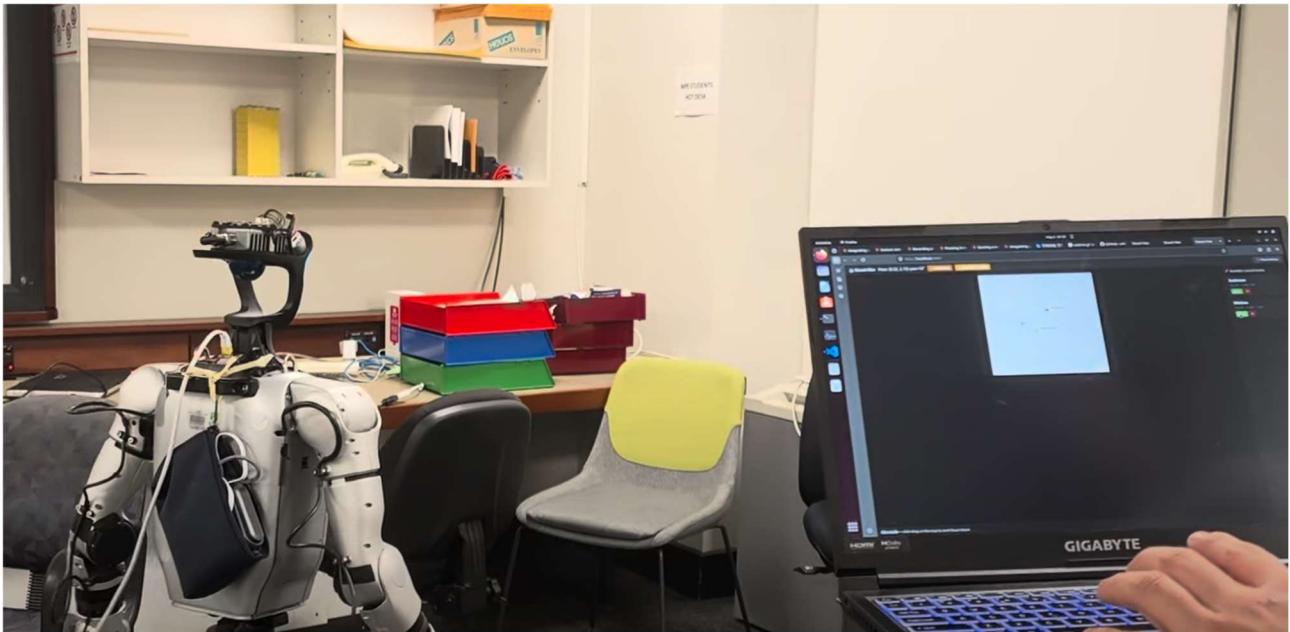
Figure 5.2.3.2. web_nav_gui map use during testing, where global-frame coordinates are input and the robot navigates to the target coordinates and bearing.
