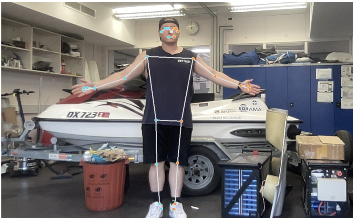
Figure 2.5: MediaPipe pose landmarking running on RGB-D camera feed.
