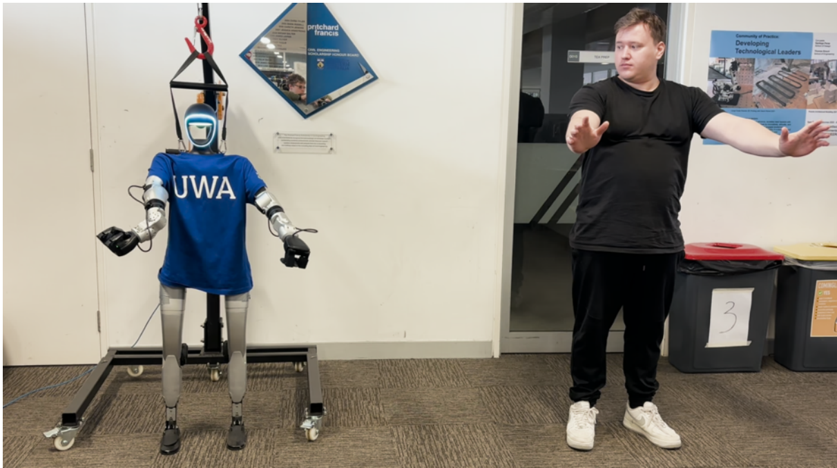
Figure 3.6: Example of arm basis collapse due to wrist-elbow occlusion.
