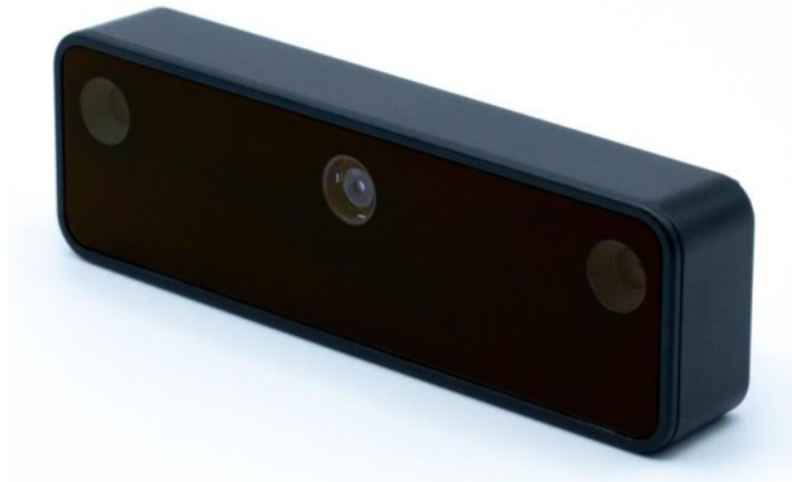
Figure 2.2: Luxonis OAK-D Lite RGB-D camera.
