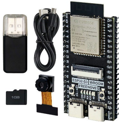
Figure 8: ESP32-S3 FREENOVE WROOM Board
