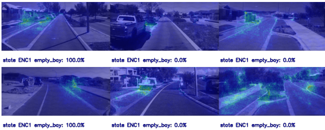
Fig. 8: Comparison of saliency maps across classification models in different driving scenarios. States ENC1 denotes EfficientNetV2SC1. empty_bay indicates the neural network empty bay classification probability output.
