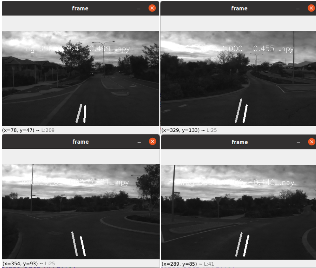
Fig. 2: NN workflow showing steering angle and throttle control commands in the test dataset. (gray line on the left represents actual commands, white line on the right represents neural network commands, line length is controlled by throttle, line angle is controlled by steering)
