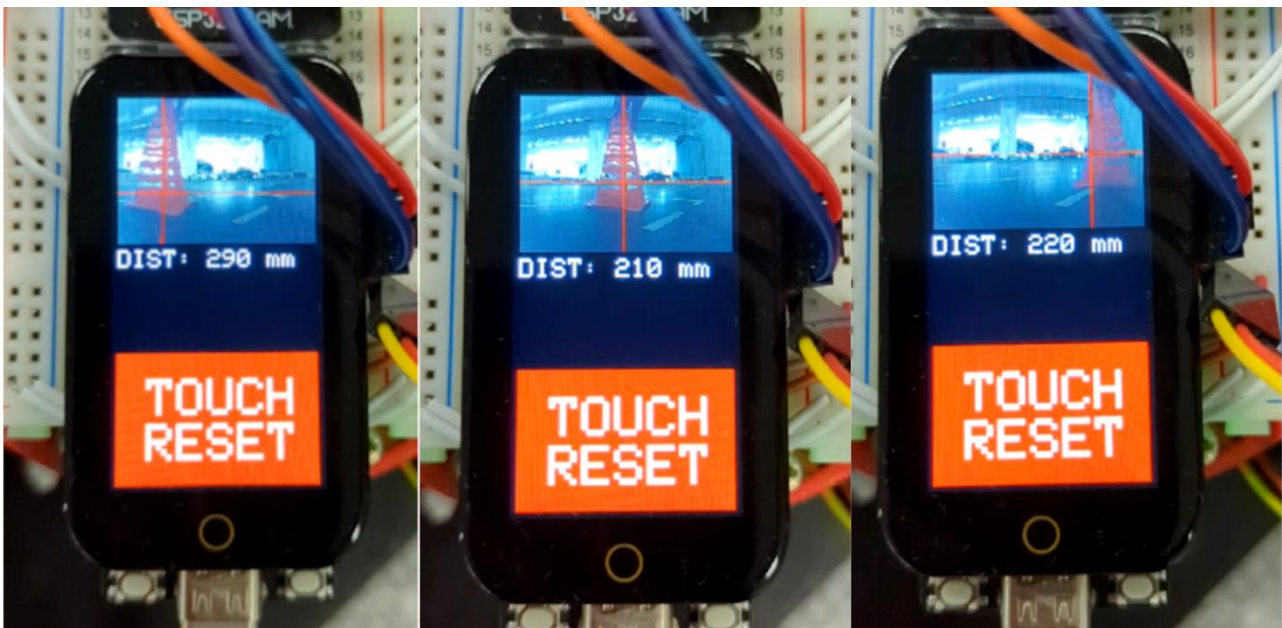
Figure 10: Sequence of images captured from a video of the Colour-Tracking Navigation program's seeking phase. In each image the red crosshairs are positioned over the orange cone, due to the colour threshold being set to detect the cone's colour.
