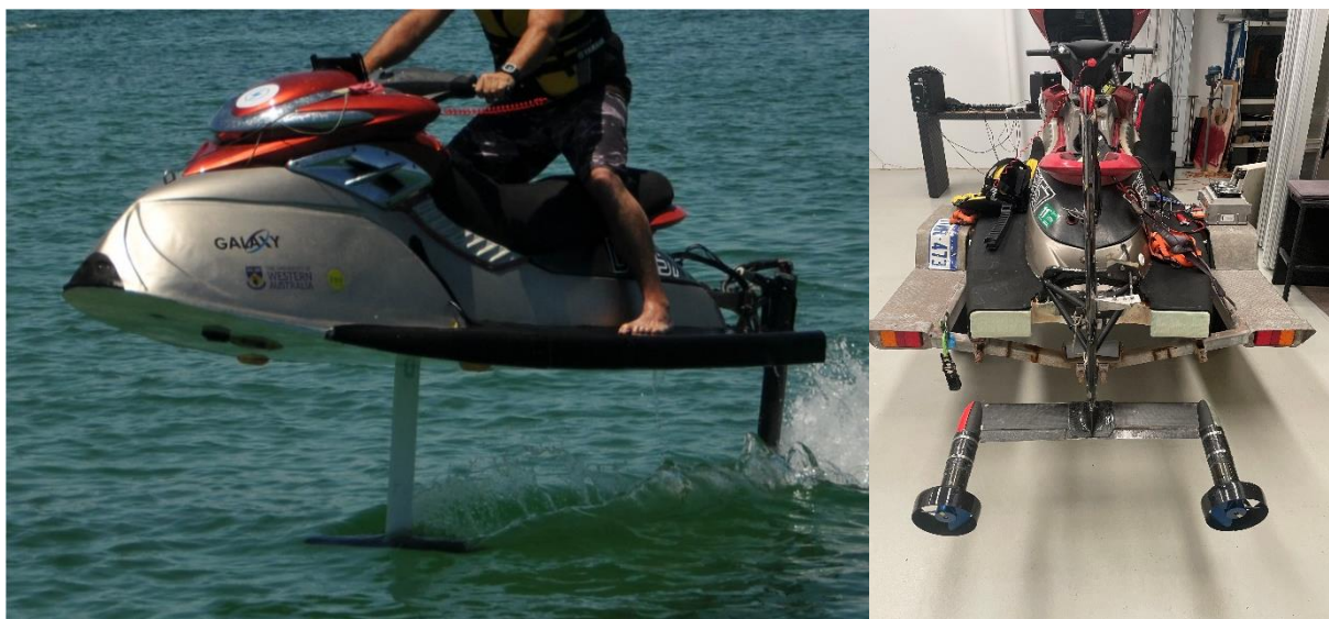
Figure 1a – Hydro-Ski successfully foiling above the water, Figure 1b rear foil assembly
