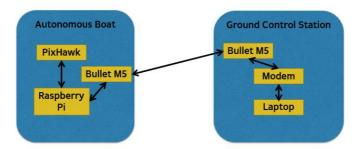
Figure 2: Communication System of Solar Boat
