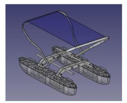
Figure 1: Twin Hull Design of Solar Boat [2]
