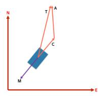
Figure 7 Vector Diagram of Apparent Wind Measurement
