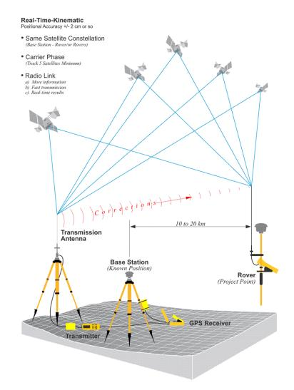
Figure 3.2: Real Time Kinematics for improved GNSS accuracy. Adapted from [14].
