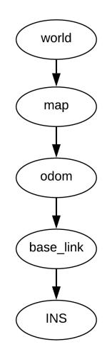
Figure 5.1: Required transform tree
