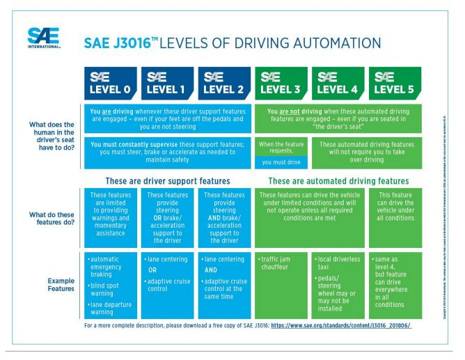
Figure 1.2: The SAE J3016 standard for driving automation. Adapted from [3]
