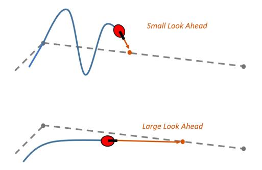
Figure 6.3: Impact of lookahead distance on the controller. Adapted from [38].
