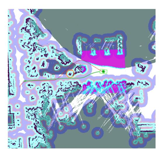
Figure 6.1: Generated path avoids the optimal route because of overhanging tree branches mapped as obstacles
