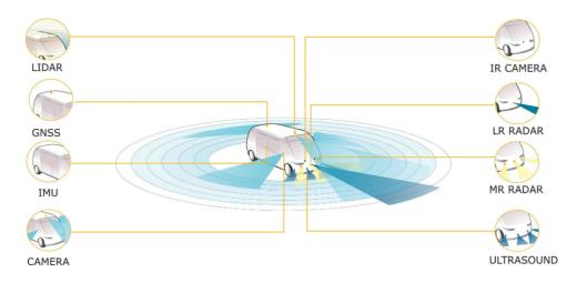
Figure 3.1: Autonomous Vehicle Sensors. Adapted from [4]
