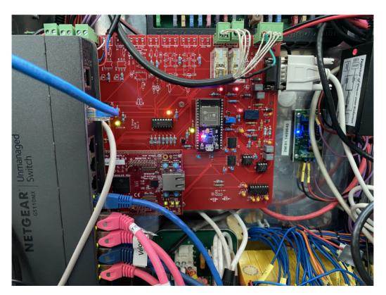
Figure 1.4: Interface board that emulates manual joystick control. Adapted from [10]
