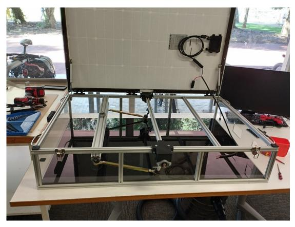
Figure 21: Image showing the chassis frame complete with acrylic side panels and solar panel lid.
