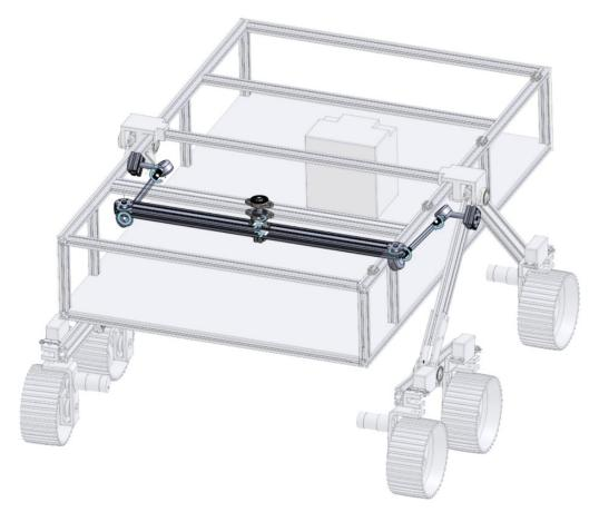
Figure 12: The differential bar mechanism highlighted on the rover model.
