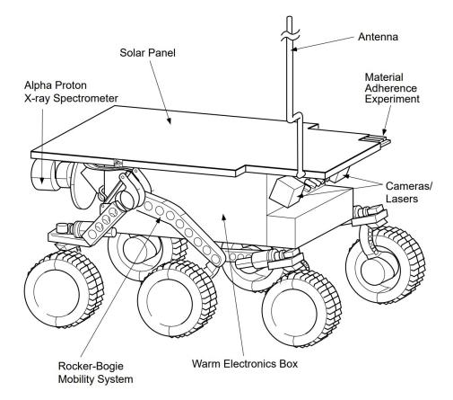
Figure 2: A concept drawing of the Sojourner rover. [10]
