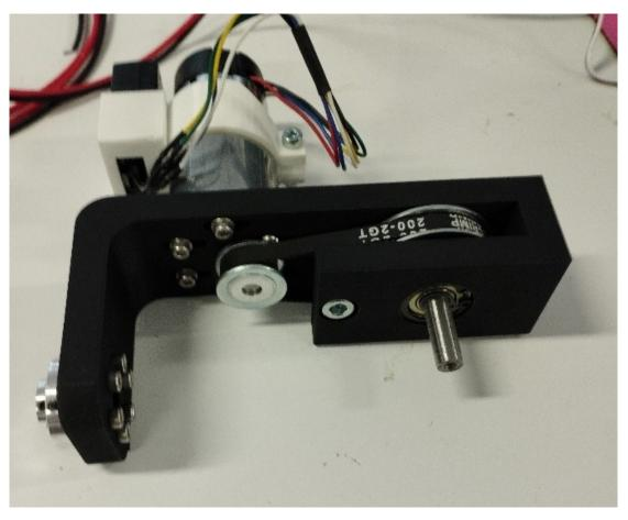
Figure 24: One of the six belt drive assemblies.
