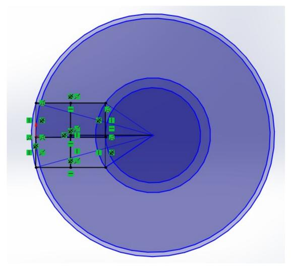
**Figure 33:** The SolidWorks sketch used to calculate the motors speeds and turning angles for swerve steering.
