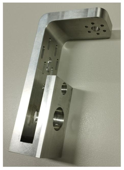
Figure 27: One of the six wheel mounts.
