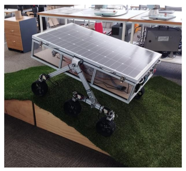
Figure 35: Image of the rover on the ramp during the slope drive test.
