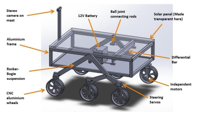
Figure 11: Initial concept SolidWorks drawing.
