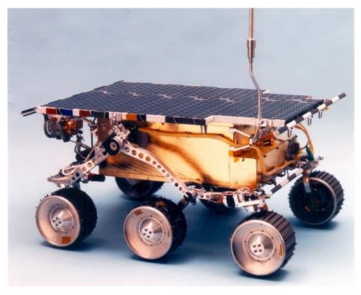
Figure 3: A photograph of the Sojourner rover a few days before launch. [11]
