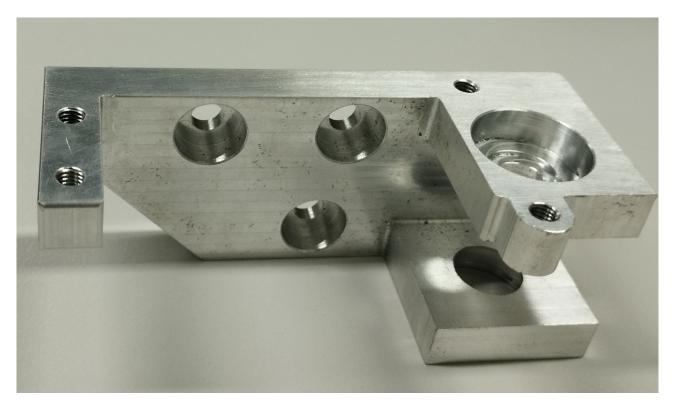
Figure 29: The one of the three inverted servo mounts.
