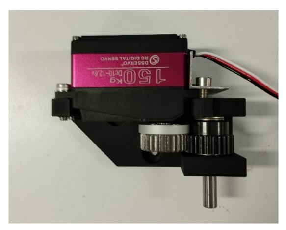
Figure 25: One of the six steering assemblies.
