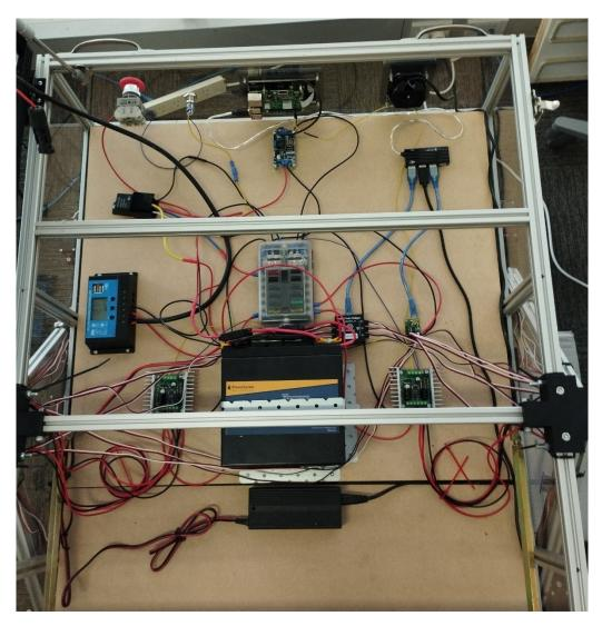
Figure 22: Top view inside the chassis after completion of all wiring.
