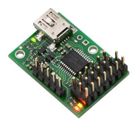
Figure 17: Micro Maestro 6-Channel USB Servo Controller [27].
