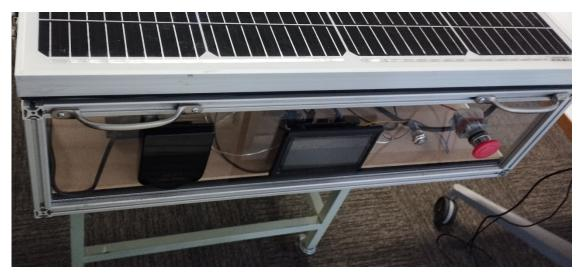
Figure 23: View of the back of the rover with the Raspberry Pi screen, buttons and charging plug mounted.
