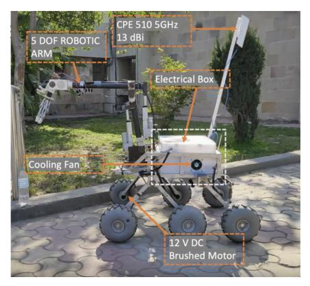
**Figure 9:** *Image of the rover built by V. Sharma, S. Sangwan and K. S. Bora at Delhi Technological University* [18].
