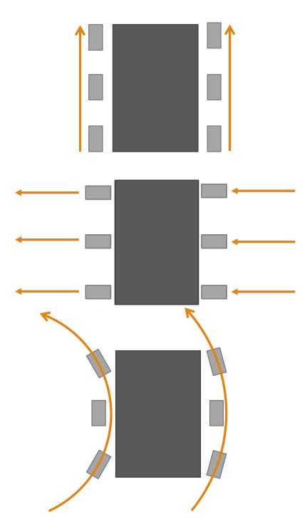
**Figure 32:** *An illustration linear driving, side driving, and swerve steering.* 32
