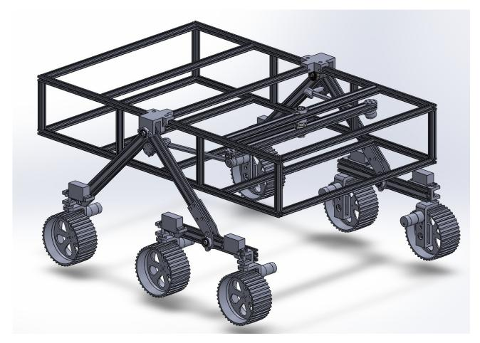
Figure 18: Detailed SolidWorks assembly of the rover.
