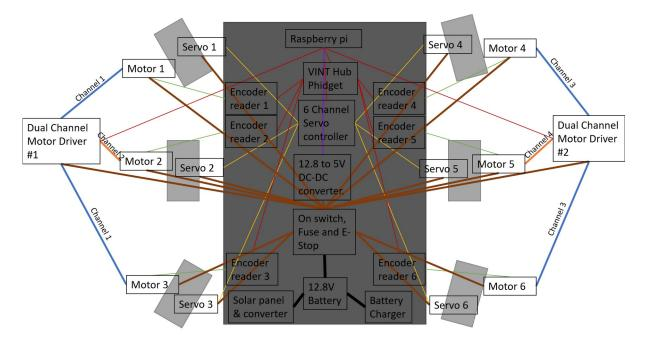
Figure 19: Planetary Rover Component Connection Diagram.
