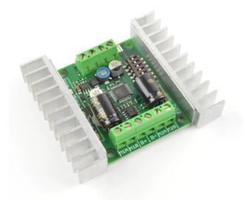
Figure 15: Sabertooth Dual 12A 6V-24V Regenerative Motor Driver. [25]
