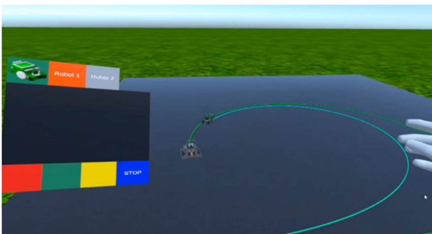
Swarm Follow -> 1 leader robot doing a circle, and a follower robot following it
