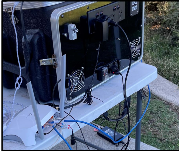
Figure 22: Wi-Fi modem used to rectify communication issues
