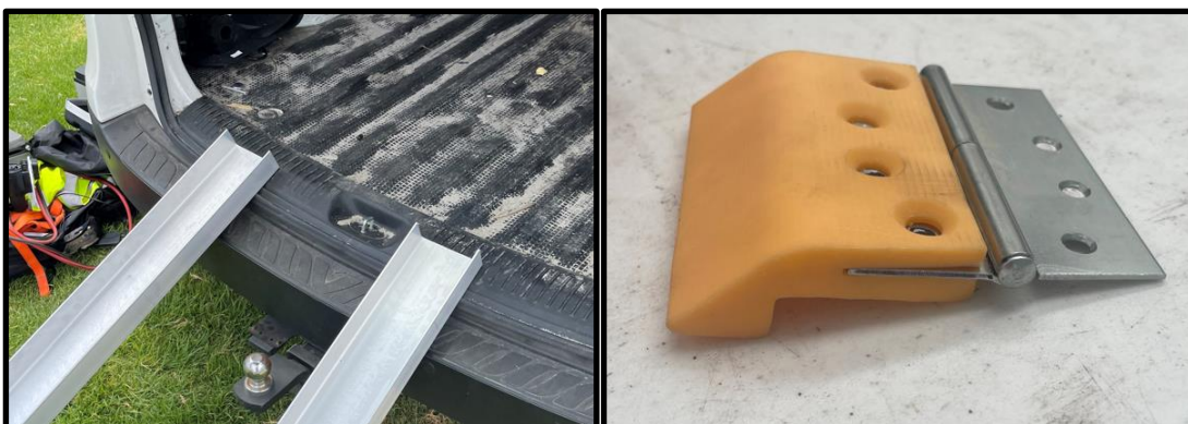
Figure 8: Proposed ramp design & 3D printed hinge.
