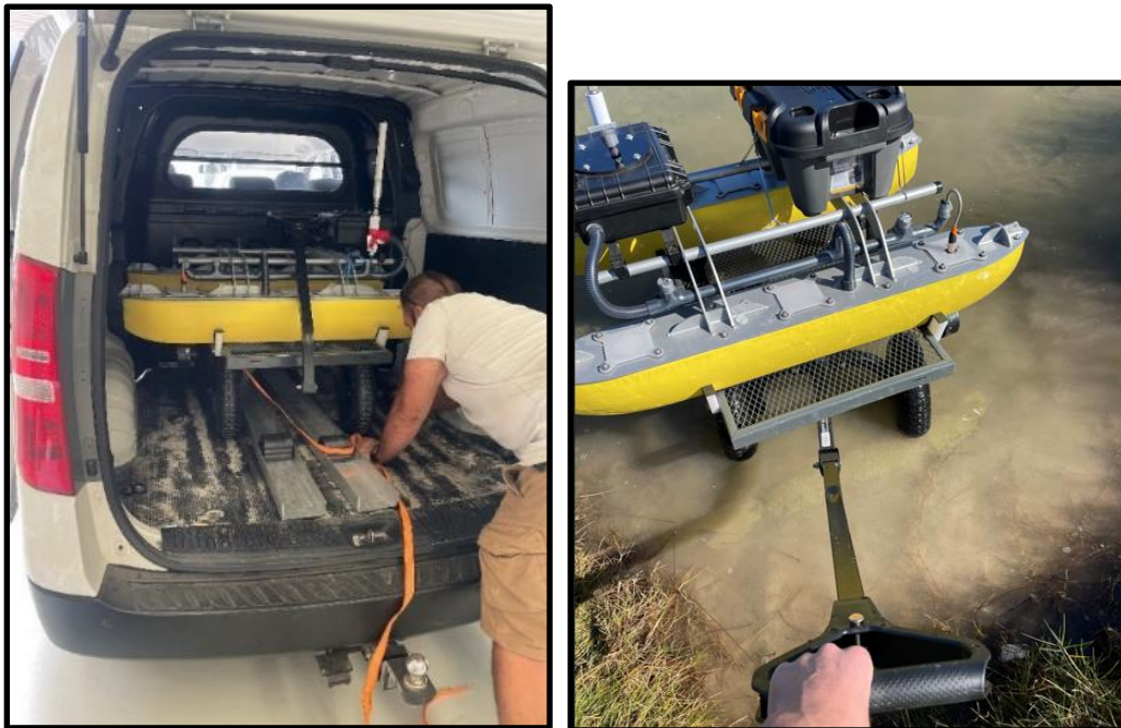
Figure 26: The carrier cart & ASV fitting within the constraints of the van & the carrier cart submerged during launching of the ASV.
