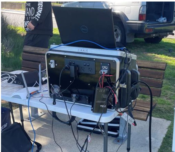
GCS - Powerpack powering multiple devices and charging using the solar blanket
