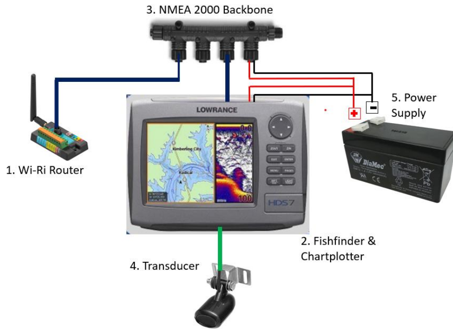
Figure 23: Bathymetric sensor network using the NMEA2000 protocol.
