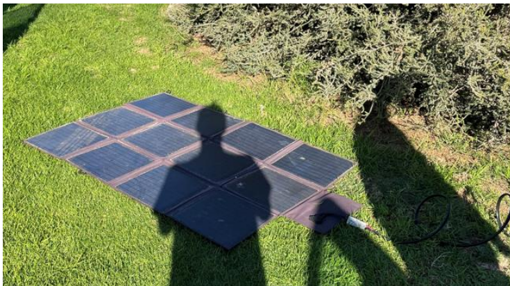
Solar Blanket used to charge the GCS - Power Pack
