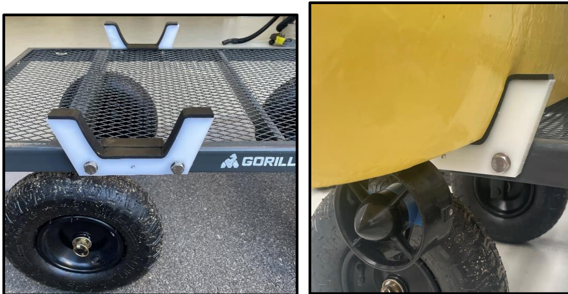
Figure 7: Saddle connection to cart & fit with ASV.
