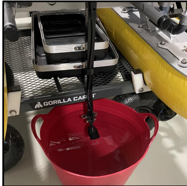
Figure 25: Connection of the transducer to the rear of the ASV.
