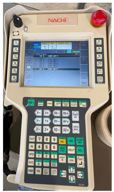
**Figure 8 Nachi Controller's Teach Pendant.** It's the main point of communication for the manual and automatic control of the Nachi robotics manipulator. It enables writing, testing, and execution of all programs. Display shows Program #25 and Step #6 is highlighted (in focus).
