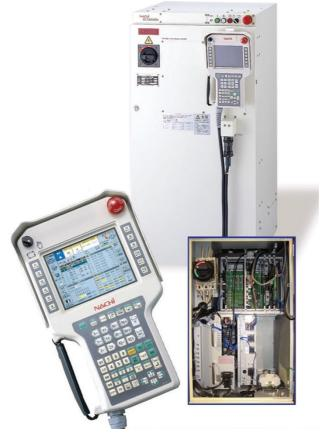
**Figure 2 Nachi AX20 Controller with the Teach Pendant ("Nachi Controller").** Nachi Controller is used to provide power to the robot and to control every aspect of the robotic manipulator. Nachi Controller have the following functions: manual control, software limits, program creation, program conversion, program execution, IO signals, etc...
