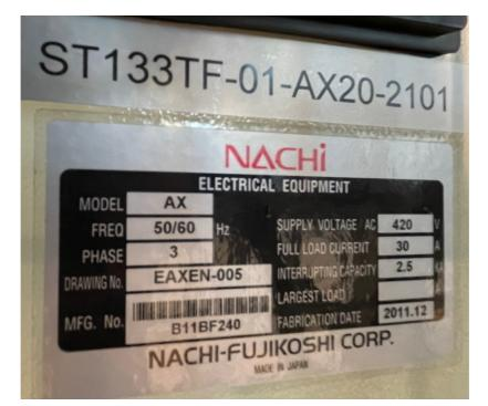
Figure 7 Power specification and Nachi Controller's model number. Nachi system (Nachi and Controller) runs on 3-phase, 420 volts and 30 amps of current.
