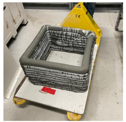
Figure 21 Final Concrete 3D Print with the Nachi robotics manipulator. After many attempts and overcoming challenges, the "Concrete 3D Printing" project were successful.
