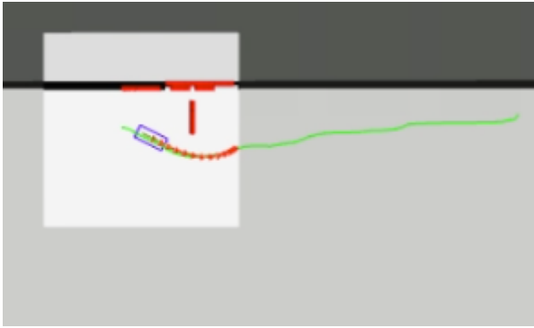
Figure 30: RViz showing the morphed path that TEB generates upon obstacle detection
