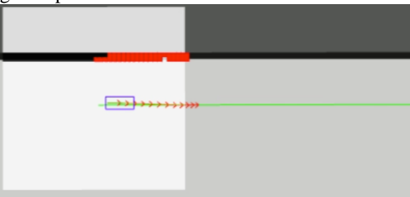
Figure 26: RViz showing straight line driving using TEB
