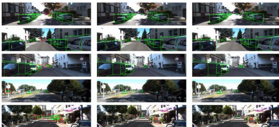
Figure 5 Sample 3D detection on KITTI dataset, from [13]
