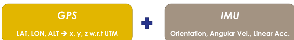
Figure 17 Odometry using GPS and IMU
