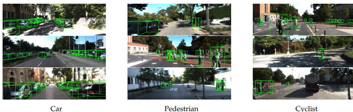
Figure 7 Sample 3D detection on KITTI dataset, from [15]
