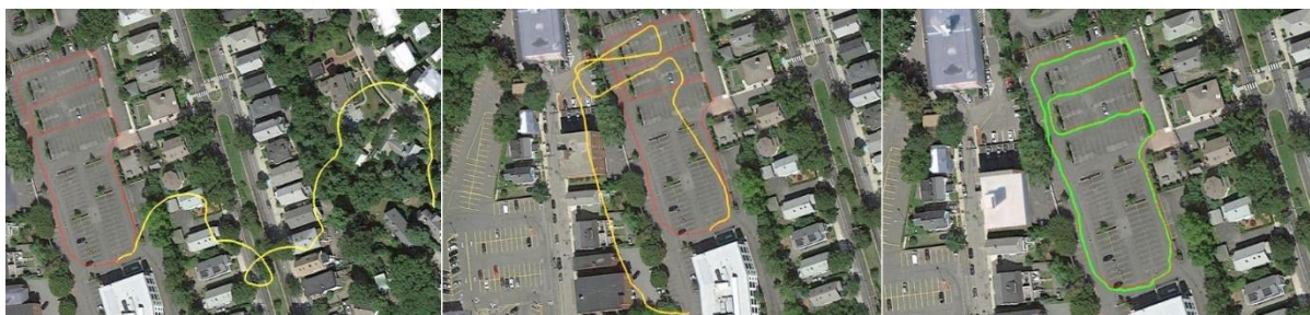
Figure 4 Output of “robot_localization” (yellow/green) using only wheel encoders (left), encoders with 2 IMUs (centre), encoders with 2 IMUs and 2 GPSs (right) against GT shown in red, from [11]
