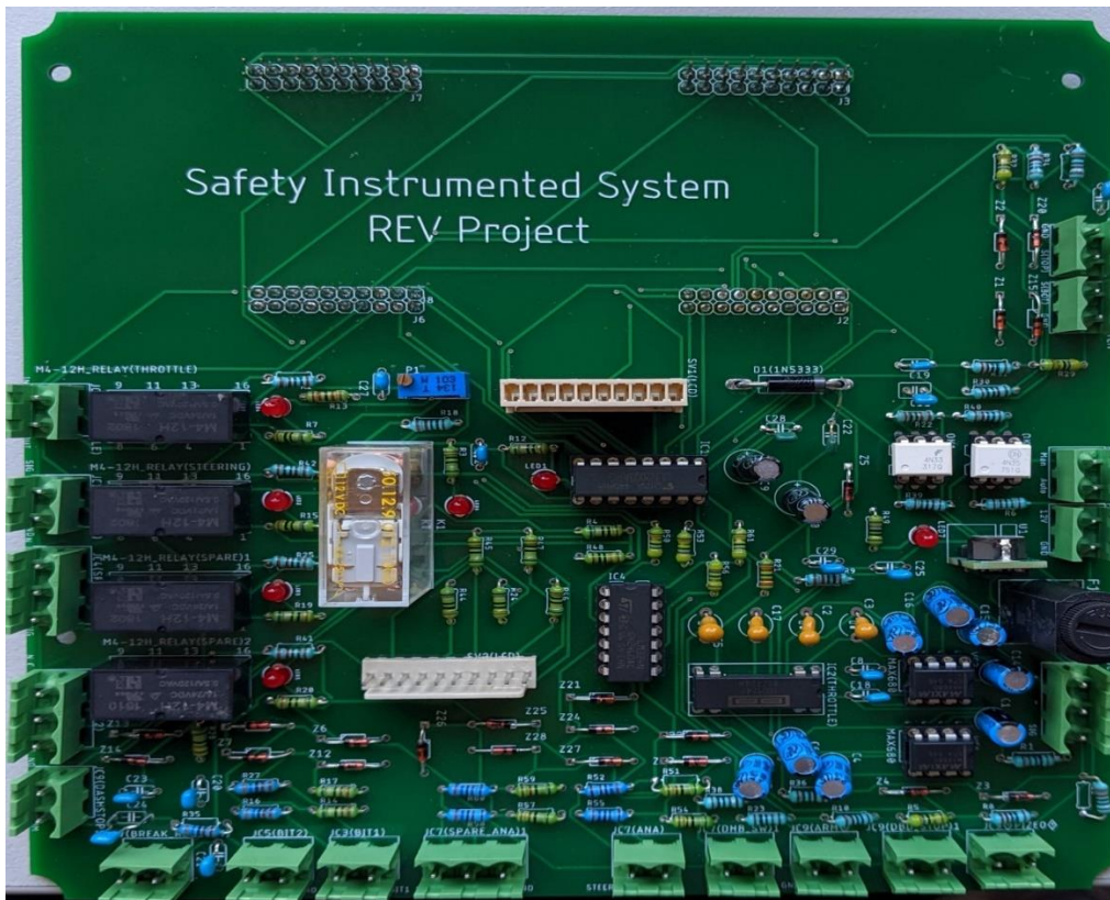
Figure 16: Safety supervisor PCB
