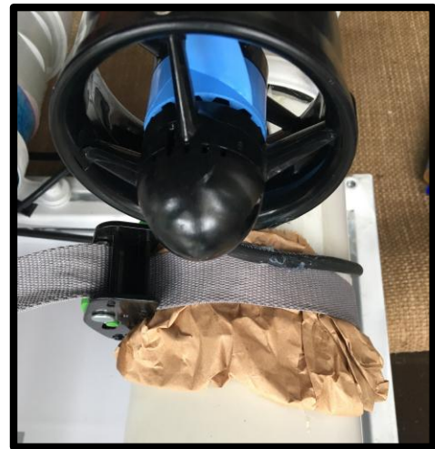
Figure 12: Thruster Fixed While Epoxy Sets
