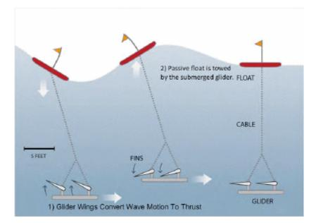
Figure 7: Description of Wave Glider propulsion
