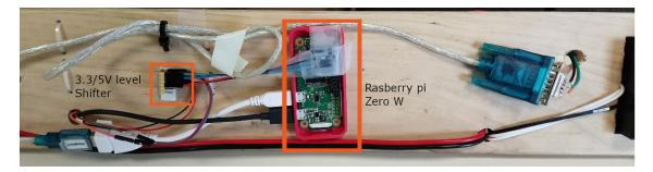
Figure 3: New hardware components
