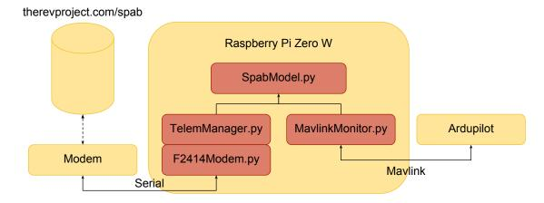
Figure 5: Client Server Architecture
