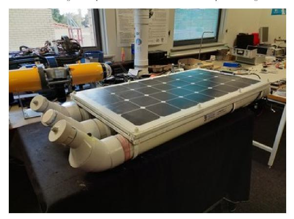
Figure 1: The UWA Solar Powered Autonomous Boat
