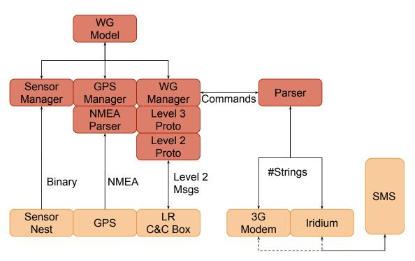
Figure 10: Wave Glider Architecture
