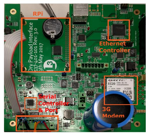
Figure 9: Payload Board Diagram
