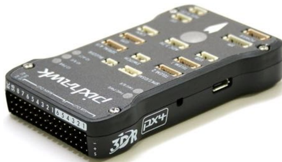
Figure 4.3: A 3DR pixhawk as used on the BlueROV2. Pixhawk is an open-hardware project and can be used for control of various devices like AUVs, Rovers or ROVs. Figure source: [60]
