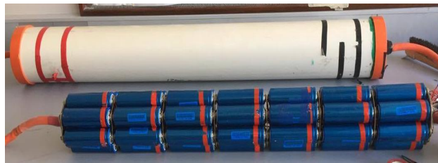
Figure 4. 7S8P battery tube used within the REVski.
