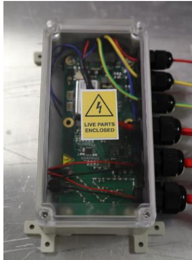
Figure 5. Photo of Bender IMD taken within the REVski laboratory.
