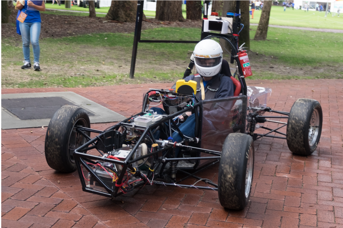
Figure 1.2.: Photo of the electric race car built by the REV-Project. The chassis of the car is in line with the rules of the Formula-SAE [SAE17]. Former members of the team converted the motors from combustion units to electrical powered, implemented drive-by-wire functionality, and way-point navigation [Dra13]. An Ibeo Lux automotive Lidar, IMU, GPS, monocular camera and wheelspeed odometry serve as the sensory body of the vehicle. Electronic actuators control steering, breaks, and acceleration.
