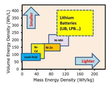
Figure 1.4: Volume Energy Density versus Mass Energy Density for various battery types (Amine, 2010)
