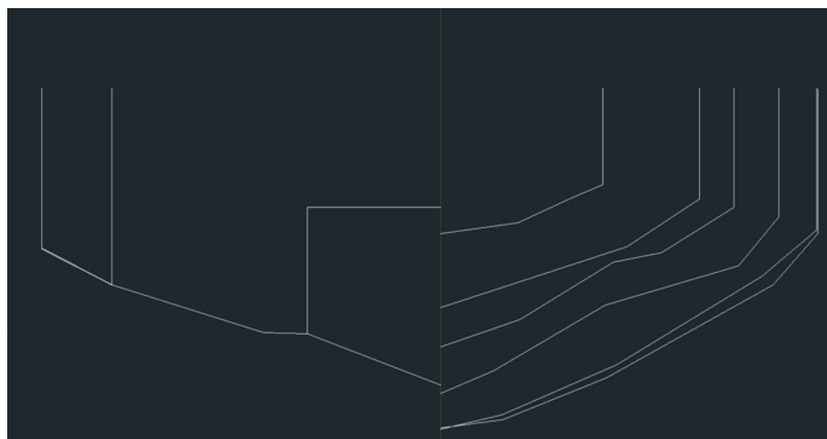
Figure 9. Body plan of REVski (Vertical axis – z axis, horizontal axis – y axis)
