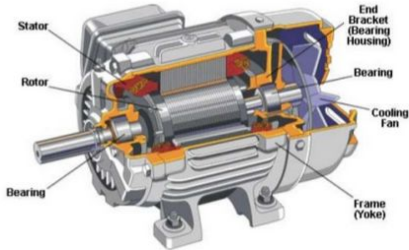
Figure 3 Asynchronous Motor Structure [7]
