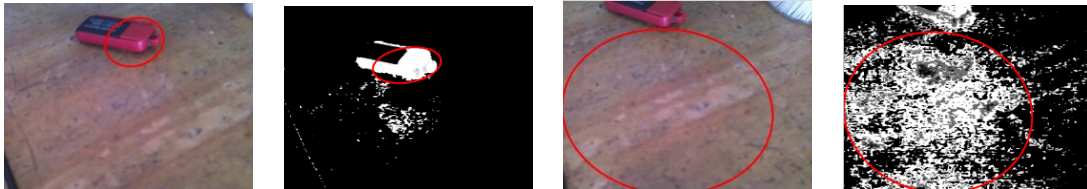
Figure 4.6: Camshift tracking, showing the back-projection image. False positive detection occurs as the tracked object is moved off-frame.
