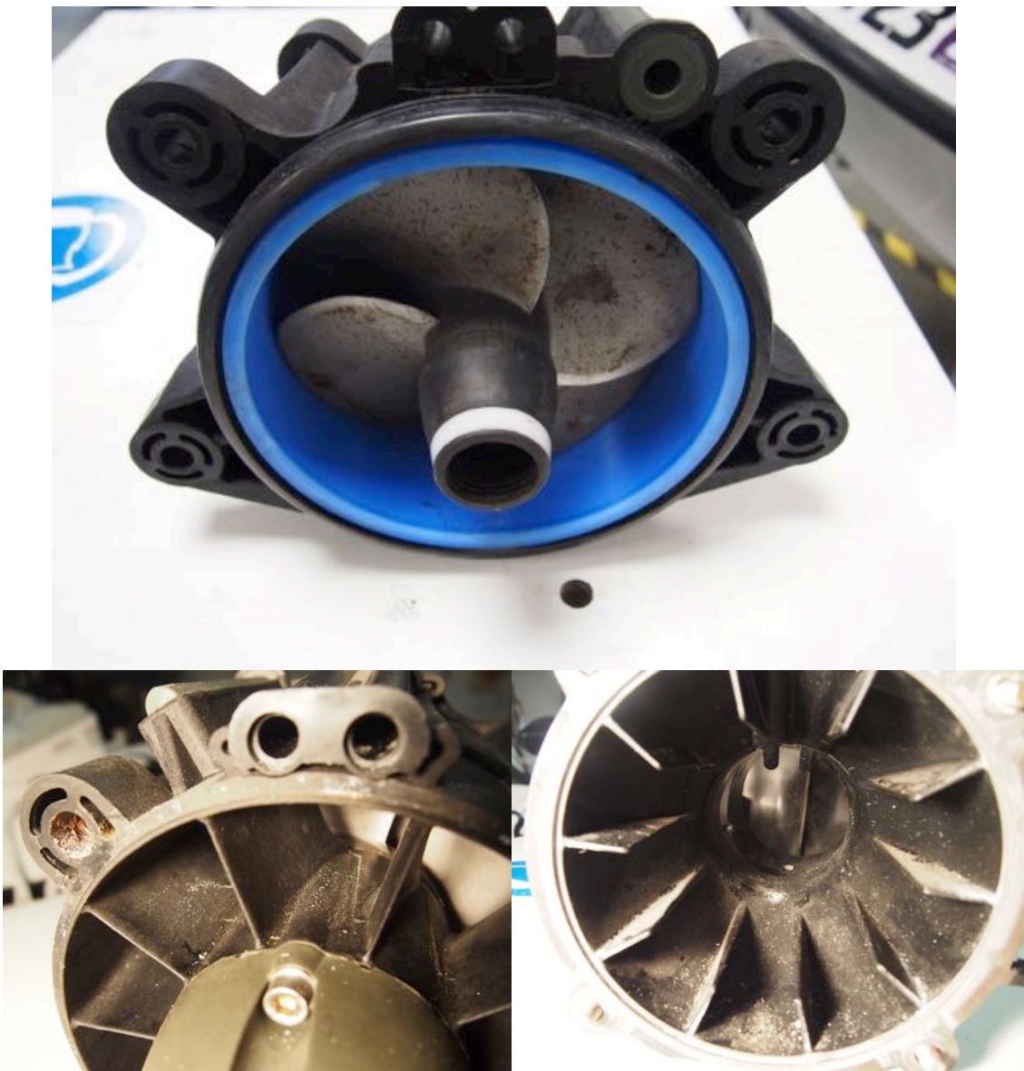
Figure 3 Clockwise from top, impeller and stator, venturi and stator outlet
