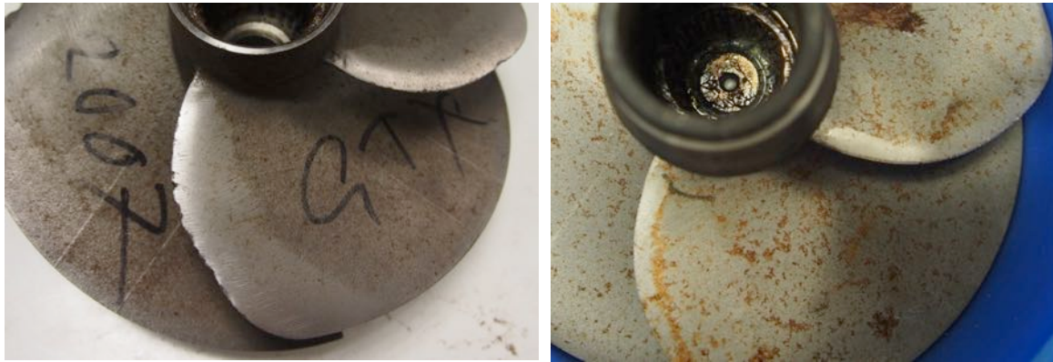
Figure 1 PWC Impellers. Left: worn impeller, Right: REV Jet impeller
