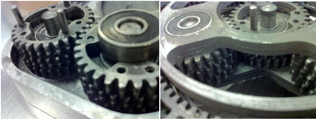
Figure 29 - (Above and below) The gears were run in after assembly. They mesh smoothly as anticipated. Some small problems with assembly occurred, especially where some laser cut components were bent out of shape due to handling. On observation, some teeth are slightly out of alignment, yet the gears mesh satisfactorily.
