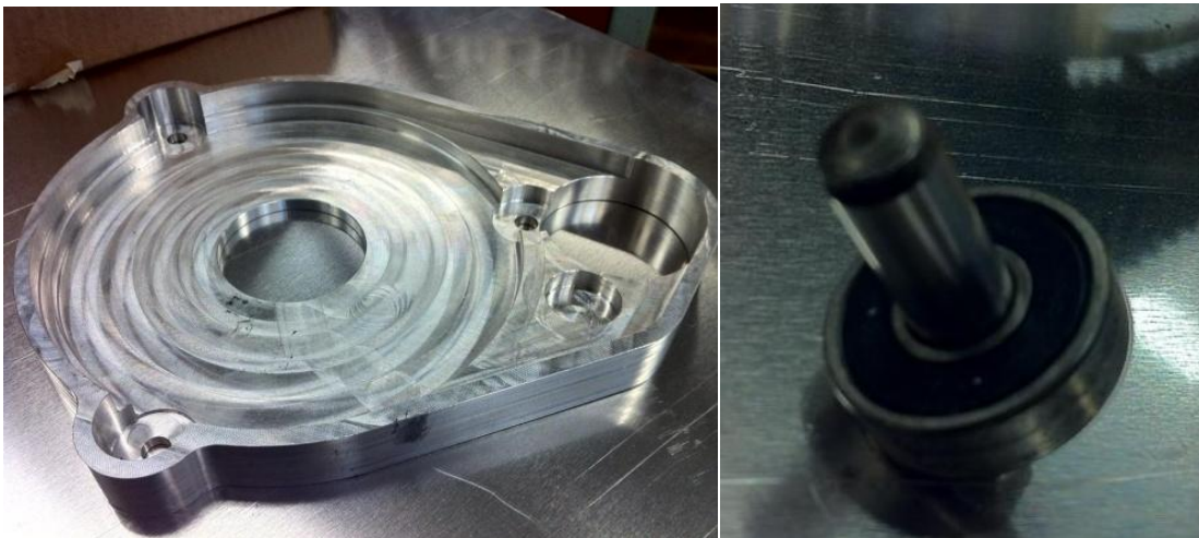
Figure 27 – (Left) The case is machined aluminium alloy, generously manufactured through sponsorship by Westurn Engineering in Mandurah, WA.
