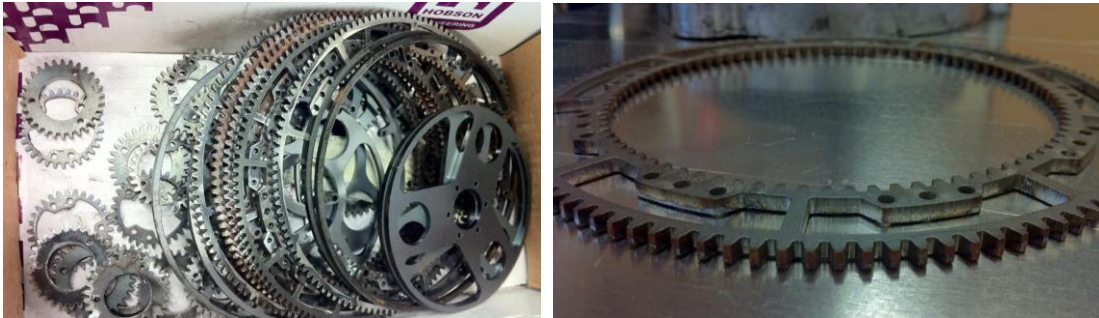
Figure 26 – The laser cut components are received. It is clear that the surface finish and geometry are both very poor. This will do fine for the short operating life expected of the device, however to minimise the probability of fracture initiation due to rough laser kerf, each gear tooth fillet was sandblasted.
