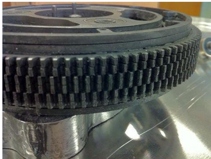
Figure 29 - (Above and below) The gears were run in after assembly. They mesh smoothly as anticipated. Some small problems with assembly occurred, especially where some laser cut components were bent out of shape due to handling. On observation, some teeth are slightly out of alignment, yet the gears mesh satisfactorily.
