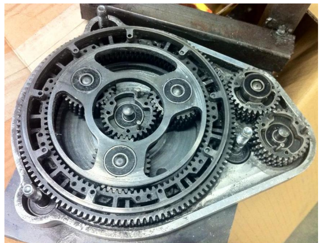
Figure 8 - The transmission unit manufactured as per the design, in a case (half of the case has been removed). It weighs only 2.33kg.
