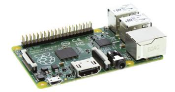
Figure 4: The Raspberry Pi Model B+ is a credit card sized computer capable of running the Linux operating system. (The Register, 2014 [64])
