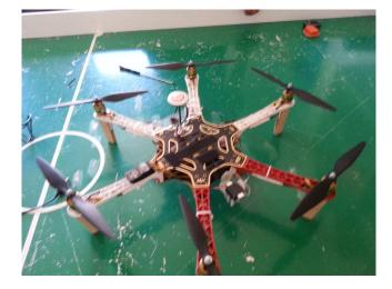
Figure 3: The hexacopter, a DJI F550 chassis modified to include a Raspberry Pi, Raspberry Pi Camera and Qstarz GPS.
