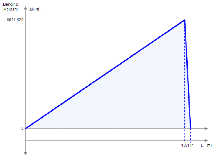
Figure 36, x-axis moment diagram for new bearing placement
