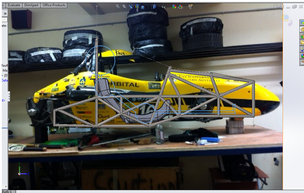
Graphic 26: Photograph transplant technique: Photograph is taken with a known dimension and transplanted into the assembly for reference. Pictured is the chassis design being evaluated with reference to the UWA Motorsport 2008 Prototype.
