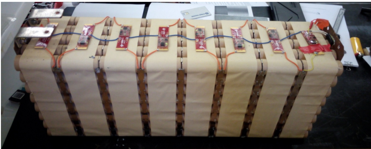
Graphic 9: The 2013 Prototype accumulator featuring permanent construction
