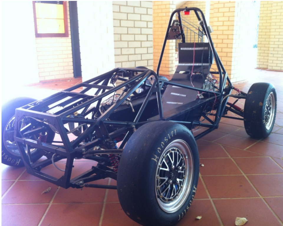
Graphic 11: The UWA Formula REV 2013 Prototype stripped of all sensitive components for welding. The vehicle features mild steel spaceframe construction. Note the locations for the two accumulators, either side of the driver.
