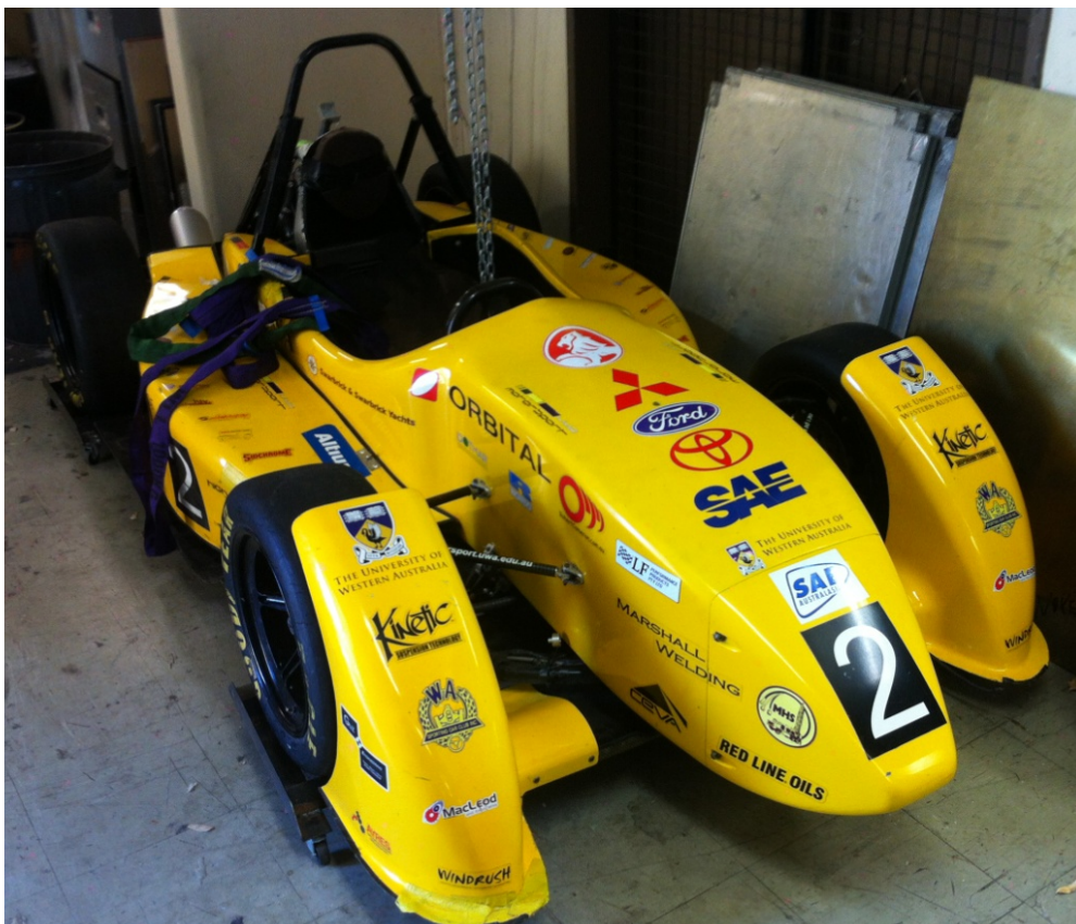
Graphic 12: The UWA Motorsport 2011 Prototype featuring carbon fibre monocoque construction.
