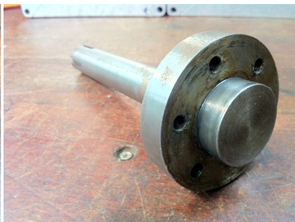
Graphic 32: EDM machined hub
