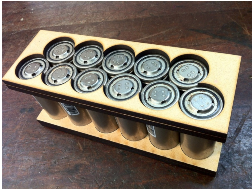
Graphic 10: The laser-cut design mocked up in wood before being approved for manufacture.
