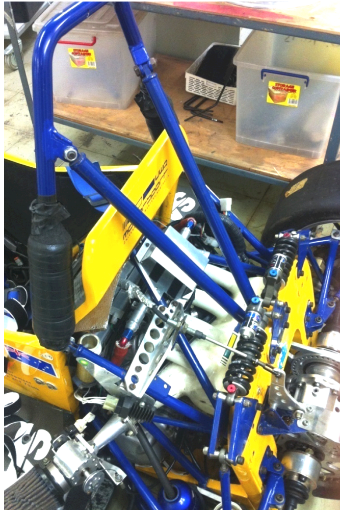
Graphic 27: The UWA Motorsport 2003 rear bulkhead was the first of its kind throughout the international competition. This vehicle was awarded the prestigious Carroll Smith Design Award for innovation in packaging.
