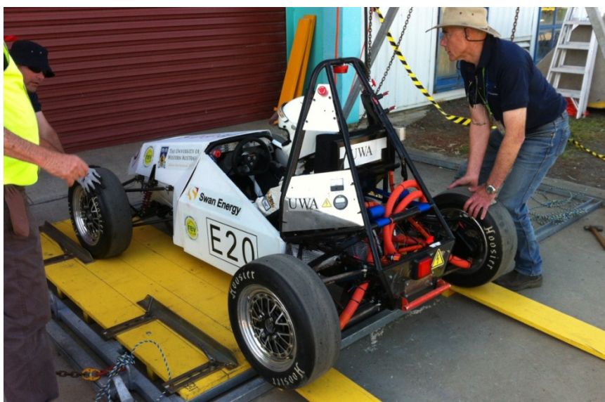
Graphic 5: The 2013 Prototype being prepared for the tilt-test: an element of the technical inspection.
