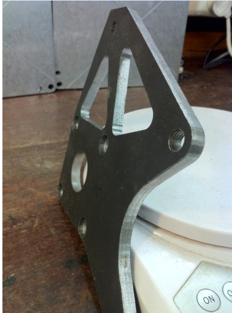
Graphic 30: Laser cut brake mount plate
