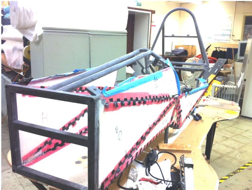
Graphic 13: The UWA Motorsport 2013 Prototype featuring hybrid carbon sandwich panel and spaceframe. This photo was taken prior to applying the carbon fibre skin.
