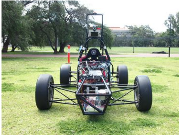
Figure 1: Autonomous Formula SAE-Electric Car
