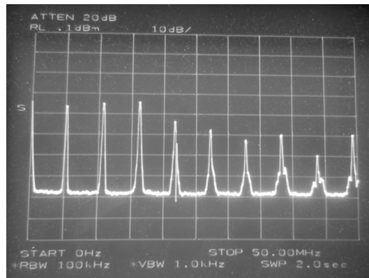
Figure 5.7: Spectrum of the RX signal from 0 to 50MHz. Remarkable are the carrier frequency of 5.5MHz and its harmonics, which are not filtered very well, causing a large total harmonic distortion which could interfere with other devices on the power line and even radiate into the air, especially when the power line is long.
