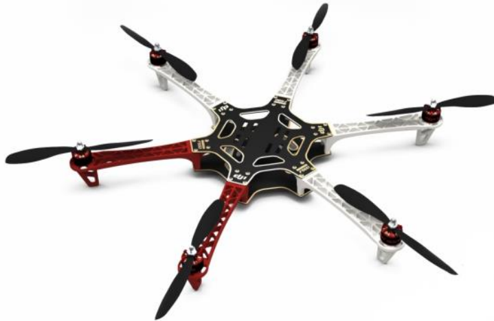
Figure 6: DJI F550 hexacopter star configuration [66]
