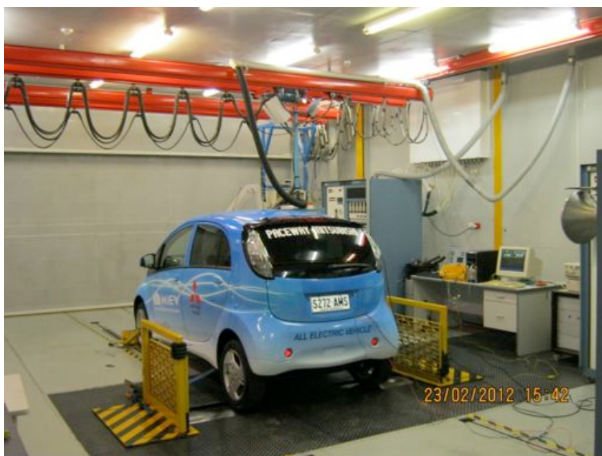
Figure 14: The Mitsubishi MiEV under testing
