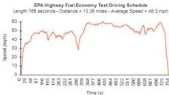
Figure 5: The second part of the US Federal drive cycle representing a driving on a Hwy [Source: [22]]
