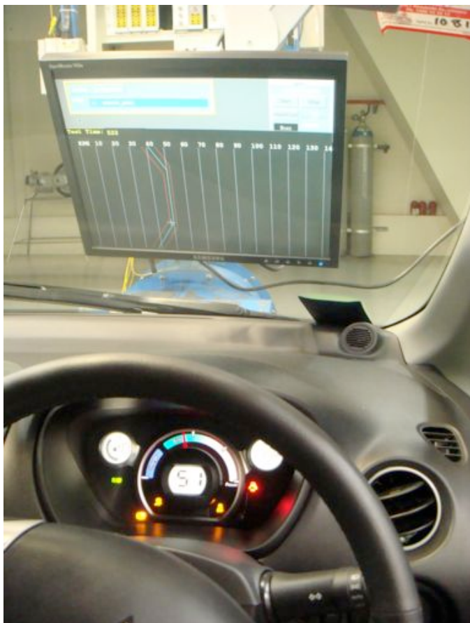
Figure 2: Computerized driving aid for a test driver required to follow a predefined drive cycle used during the testing at Orbital.
