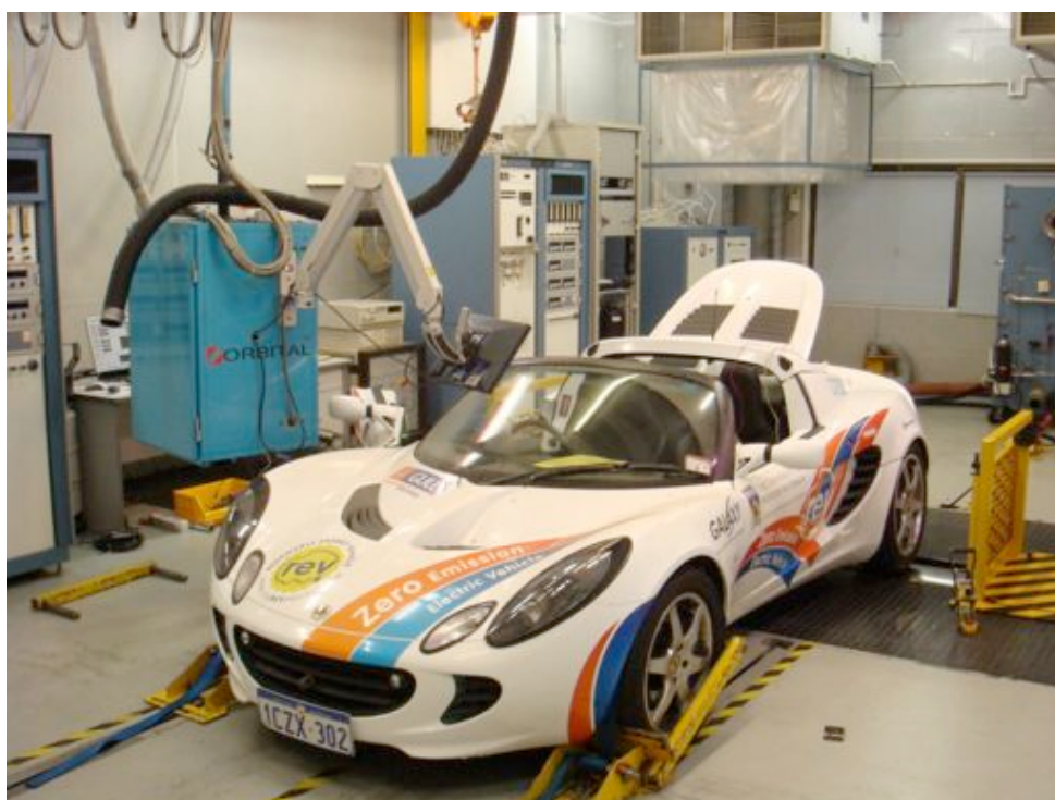
Figure 15 Lotus prepared for testing on the chasis dynamometer.
