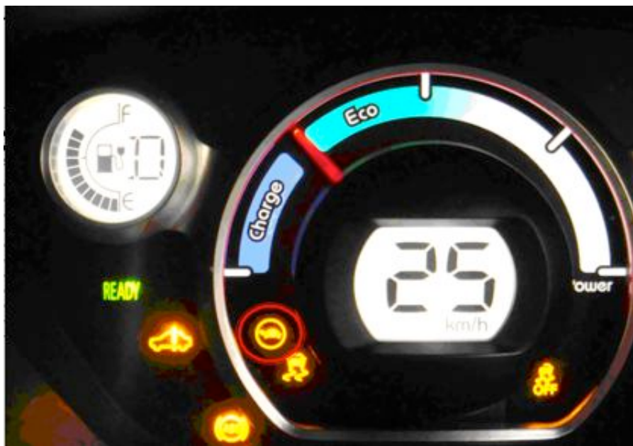
Figure 22: The MiEV dashboard informing about system errors and the limp mode indicated by the symbol of the turtle (inside the red circle)
