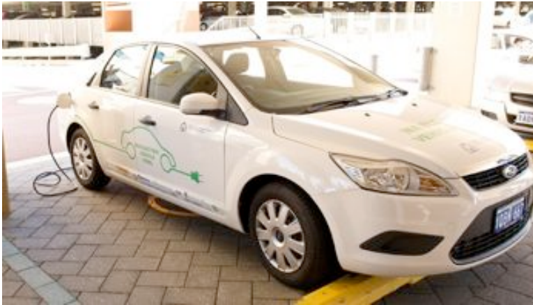
Figure 8: A Ford Focus converted EV [Source: [34]]
