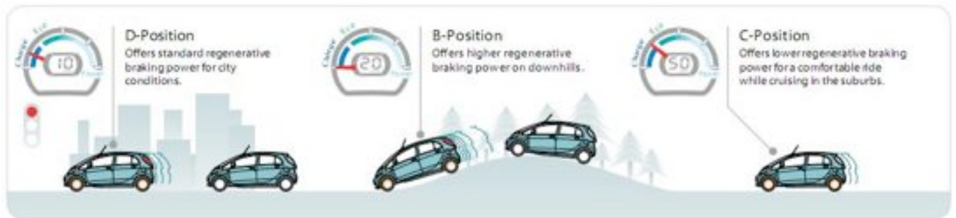
Figure 12: The driver's options for the RBS settings [Source: [32]]
