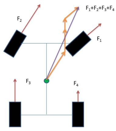
Figure 4.3: Torque Vectoring
