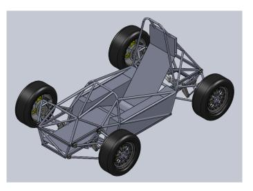
Figure 6.9: Isometric View of Chassis Design
