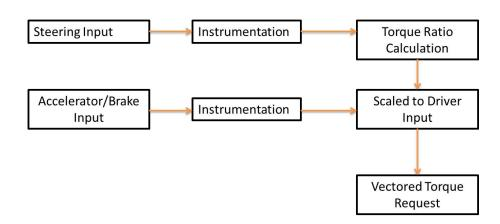
Figure 4.1: Torque Vectoring Flow Diagram
