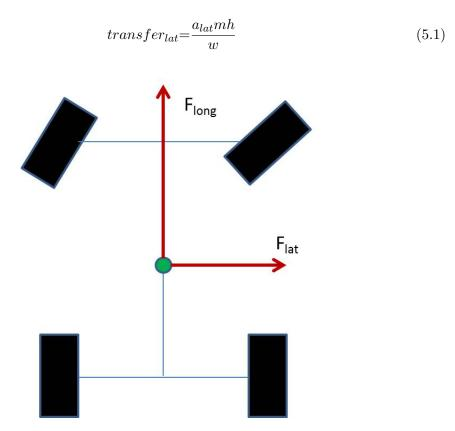
Figure 5.3: Lateral & Longitudinal Forces
