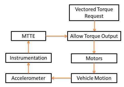
Figure 5.1: Traction Control Process
