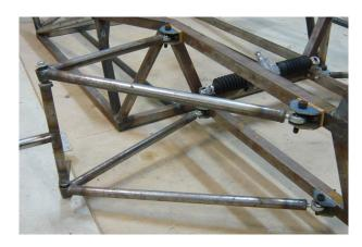
Figure 3.6: Suspension Mounts
