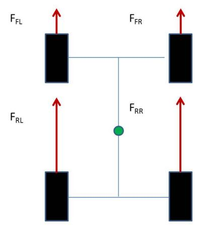
Figure 5.6: Resulting Forces using MTTE - Straight Line
