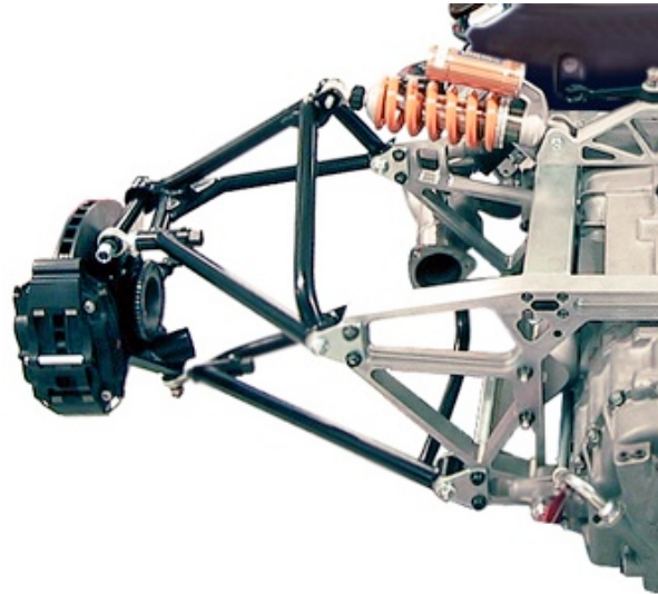
Figure 8-6: Koenigsegg upper wishbone triangulation (Solidworks Roadster 2011)
