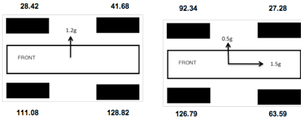
Figure 13-7: Tyre loading under 1.2g lateral acceleration and (1.5g braking combined with 0.5g lateral acceleration)
