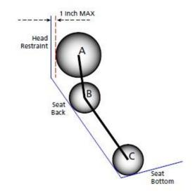
Circle A = Head with helmet – 300 mm diameter Circle B = Shoulders – 200 mm diameter Circle C = Hips and buttocks – 200 mm diameter
