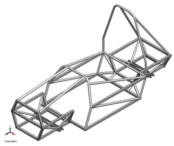
Figure 33 Front Bulkhead and forward front roll hoop supports
