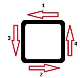
Figure 37 Order and direction welds should be made around a square tube joint
