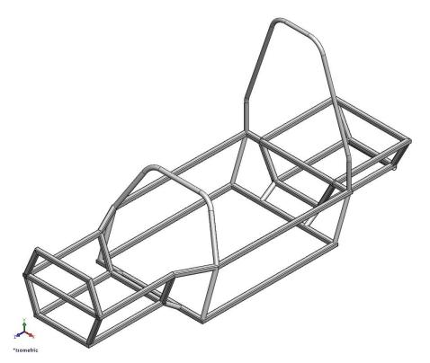
Figure 40 Roll hoops then bent into shape and added to the rest of the frame with the top section of the bulkhead
