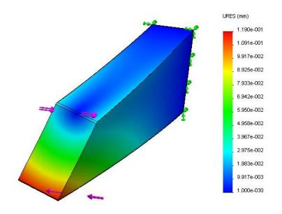
Figure 18 SolidWorks model of a single battery box in torsion
