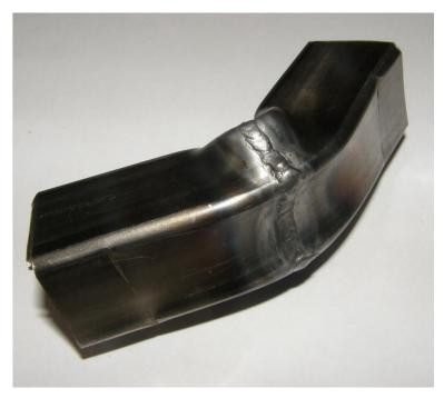
Figure 53 Three Point Bend weld sample
