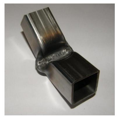
Figure 52 Three Point Bend weld sample
