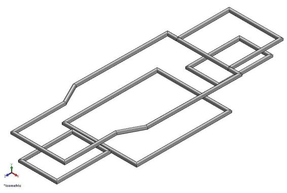
Figure 38 Horizontal Planar sections are welded first
