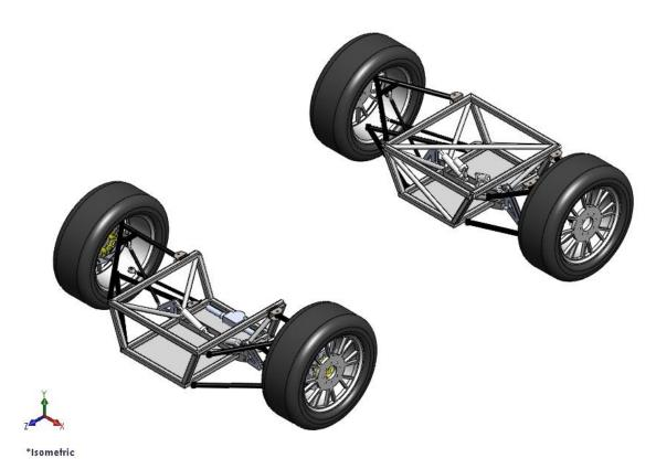
Figure 29 Front and rear chassis sections with suspension shown
