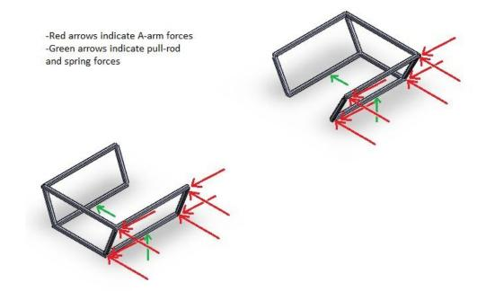
Figure 7 Basic ends of the chassis that hold the suspension arms in place. (Forces are mirrored on the opposite side of the chassis)
