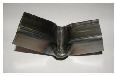
Figure 51 Three Point Bend weld sample
