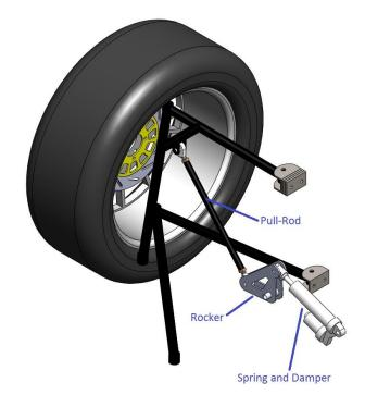
Figure 23 Front-Right suspension assembly as designed by Marcin Kiszko (Kiszko, 2011)
