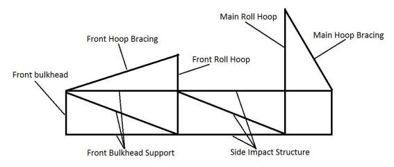
Figure 2. Pictorial representation of the members required by the FSAE rules.
