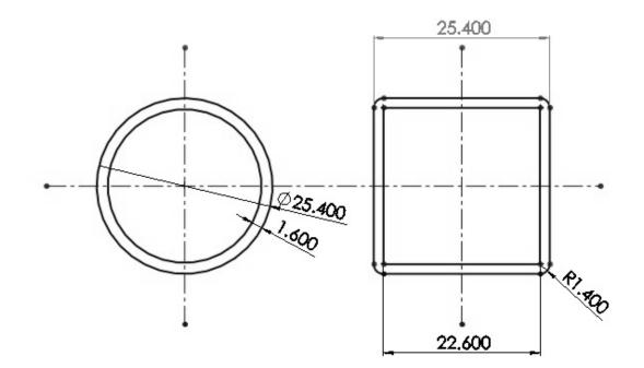
Figure 8 Dimensions of the square and round tubing used
