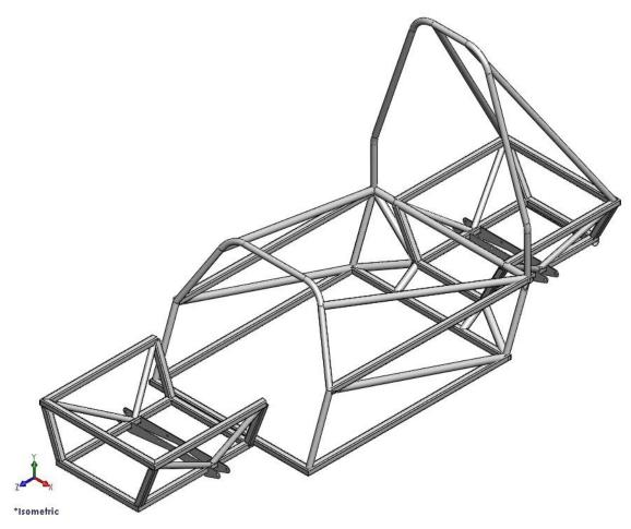
Figure 32 Front roll hoop, roll hoop supports and side impact structure now shown
