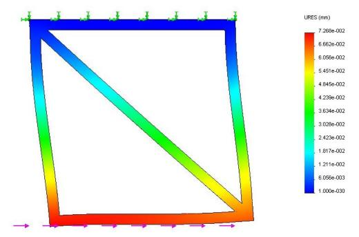
Figure 12 Displacement contour for SolidWorks model of a triangulated square frame
