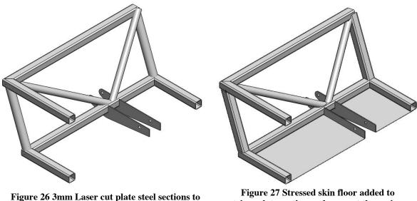
Figure 26 3mm Laser cut plate steel sections to mount spring and rocker
