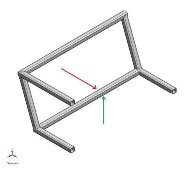
Figure 24 X and Y forces introduced into the frame by the suspension rocker
