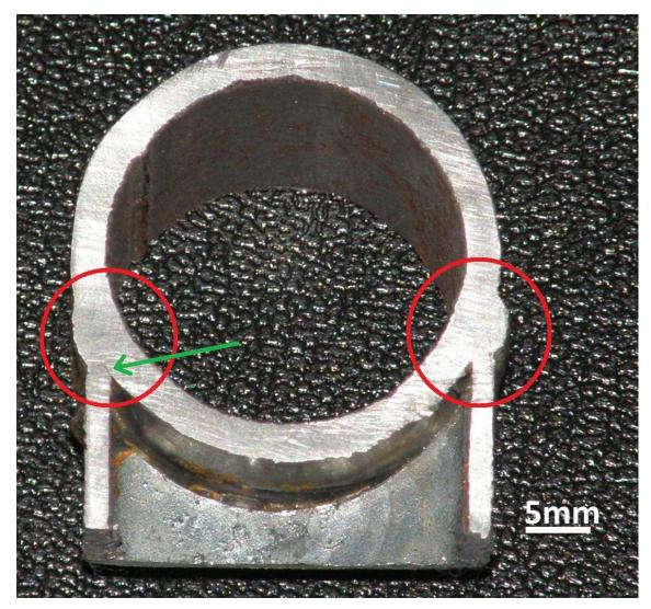
Figure 48 Weld sample square tube welded to roll hoop tubing. Incomplete fusion indicated with green arrow
