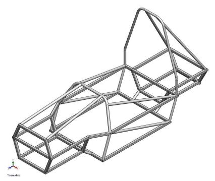
Figure 41 Roll hoop supports added along with side impact diagonal members
