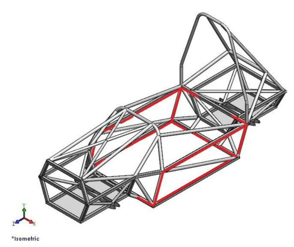
Figure 35 Battery box to frame weld attachment
