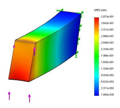
Figure 19 SolidWorks model of a single battery box in bending
