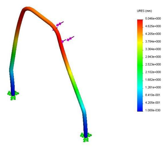
Figure 31 SolidWorks simulation of roll hoop in roll over situation
