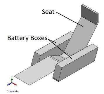
Figure 17 Stressed battery boxes and seat used to stiffen cockpit section of chassis
