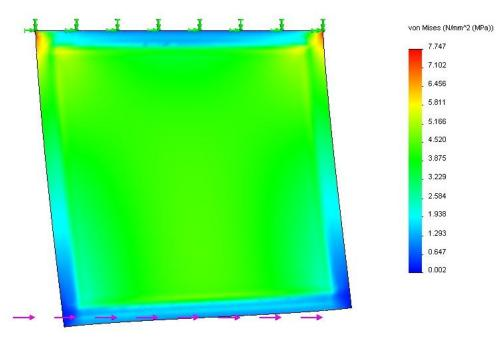
Figure 15 Von-Mises Stress contour for SolidWorks model of a square frame with stressed skin reinforcement
