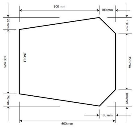
Figure 4 Cockpit entry template
