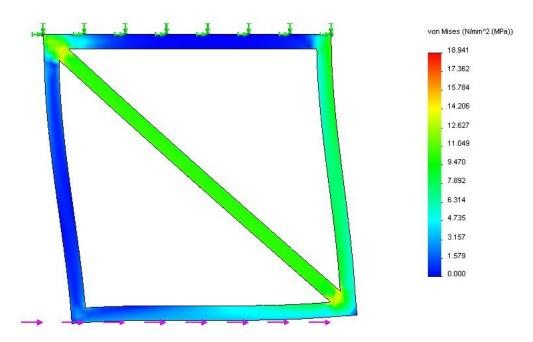
Figure 13 Von-Mises Stress contour for SolidWorks model of a triangulated square frame
