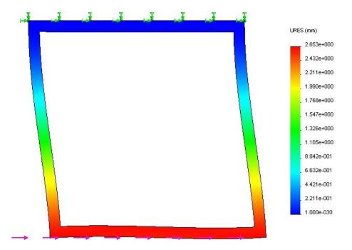
Figure 10 Displacement contour for SolidWorks model of an un-triangulated square frame
