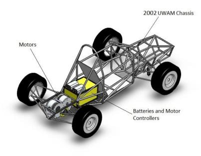
Figure 1 2001 UWAM Chassis converted to electric power using a conventional inboard engine layout
