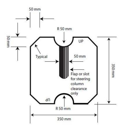
Figure 5 Foot-well clearance template
