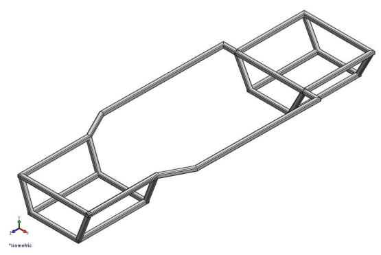
Figure 39 Front and rear lower sections attached to main horizontal section
