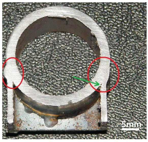
Figure 49 Weld sample square tube welded to roll hoop tubing. Incomplete fusion indicated with green arrow
