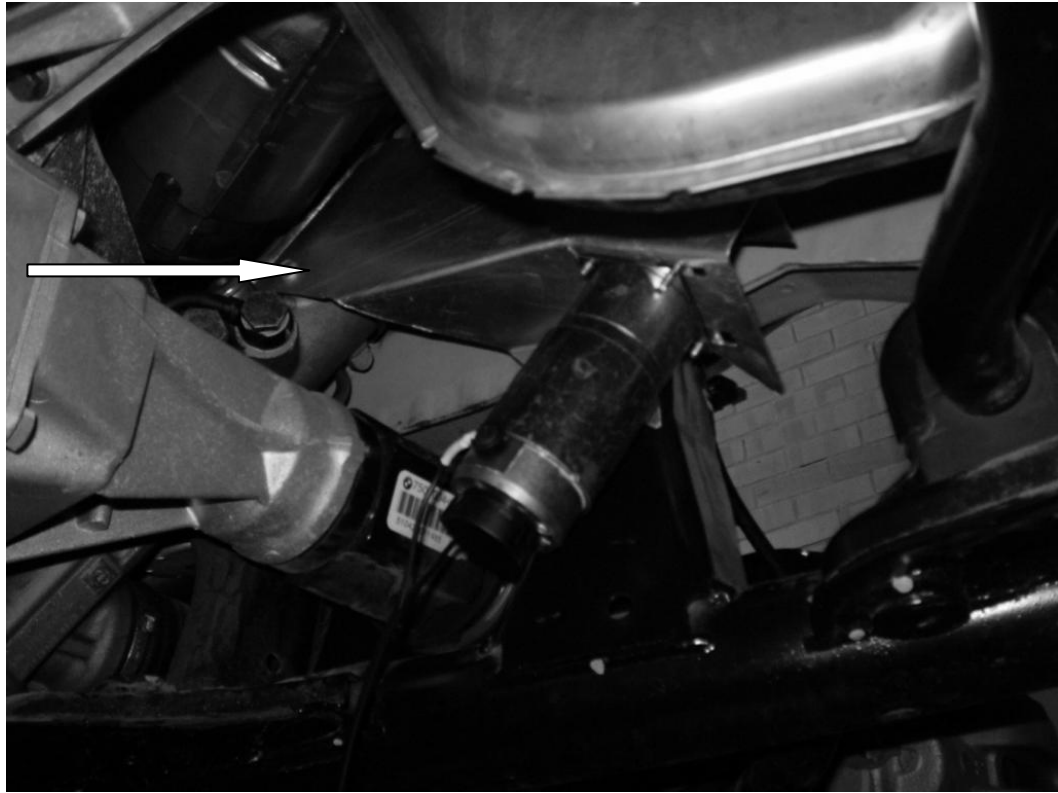
Figure 41: Installed Actuation System From Beneath Car, Steering Rack Mounting Bolt Indicated
