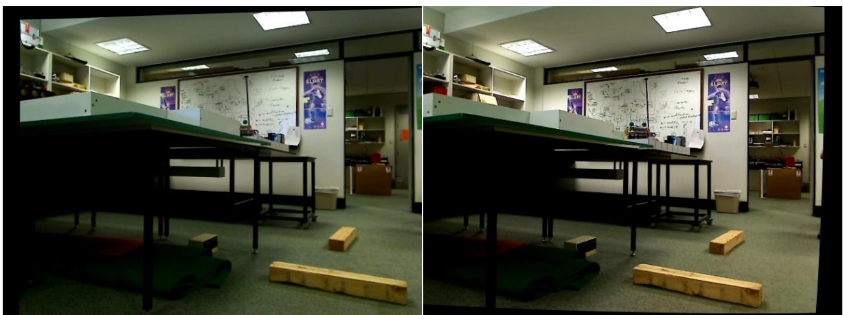
Figure 6.3 Left and right images after calibration/rectification
