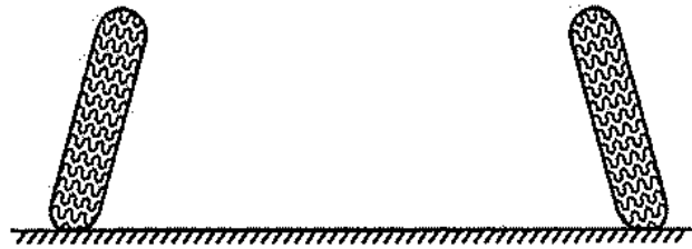
Figure 1.3: Negative camber (Milliken & Milliken 1995)
