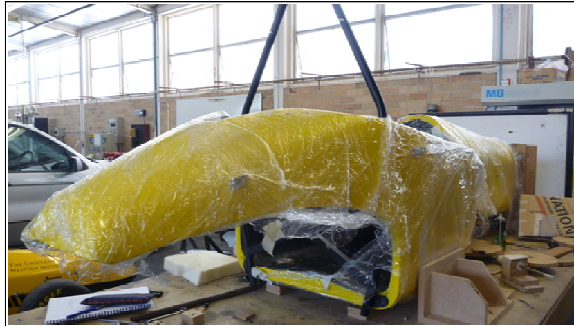
Figure 5-2: Construction of the 09 UWAM FSAE chassis.
