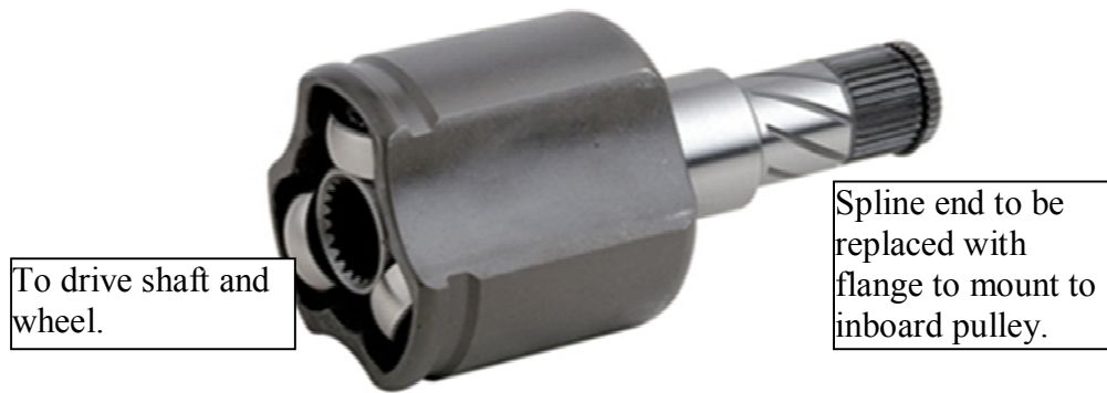
Figure 4.8-2: Inner CV joint modification. (KML Bearing 2009)
