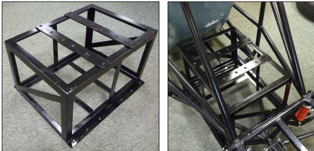
Figure 2.5-1: Left - manufactured battery cage; right – battery cage in its location behind the driver's seat.
