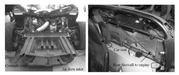
Figure 16: Lotus Elise crumple zone (left) and rear firewall behind seats (right).
