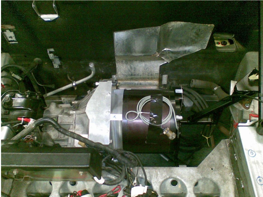
Final assembly of motor mounts
