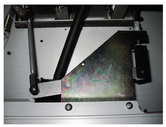
**Figure 4.2**: The accelerator system. Accelerator is in top left and the cable running to the pot box is at the top right.
