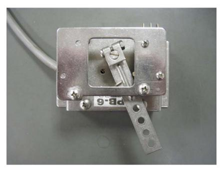
**Figure 3.7**: A pot box used to develop the 0.5-4.5 V brake or accelerator signal.
