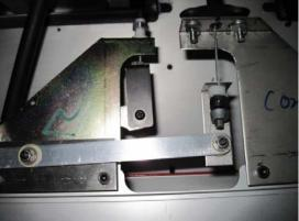
**Figure 4.3**: Images of the braking system as well as the accelerator system. All parts on the braking system were designed and manufactured for this project.
