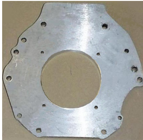
Figure 4.10: The adapter plate had been fabricated by the vertical milling machine
