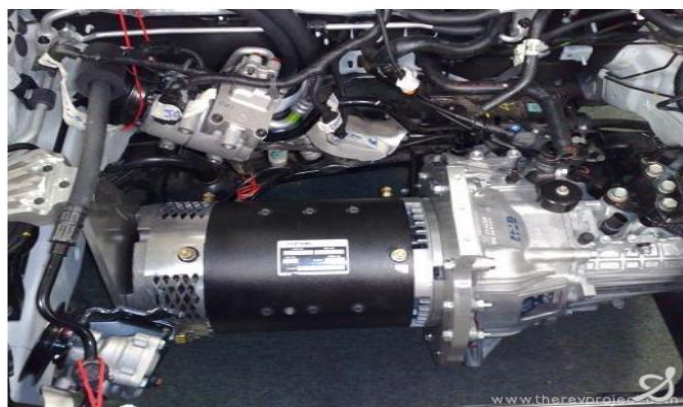
Figure 4.14 : The motor and transmission are supported by the front adapter plate and the rear support plate.
