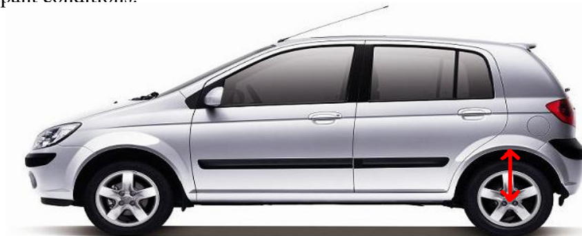
Figure 5.1: Ride height measurement
